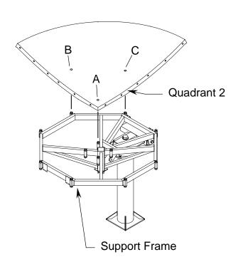
A) Position quadrant 2 (quadrant 4 for inverted) to the bottom left side of the frame as shown. Note that it may be necessary to loosen the 3 reflector inserts to attain the proper alignment with the 3 tubes in the support frame. this procedure may occur with each of the quadrants.
