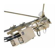
5700 transceivers antenna mounted in 1:1 configuration
