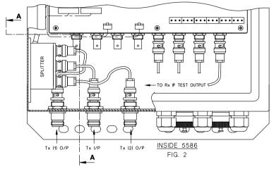
5586 Redundancy Controller
