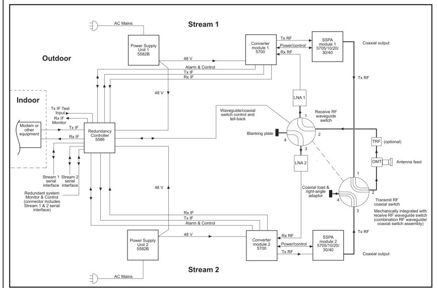
Figure power C-Band transceiver with a combined RF waveguide/coaxial switch Block diagram of the single switch redundancy system for the low
