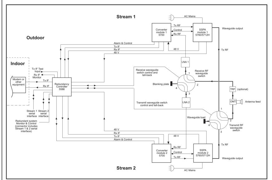
Figure power C-Band transceiver with separate waveguide switches <u>ဒ</u>-ဒ Block diagram of the dual switch redundancy system for the high
