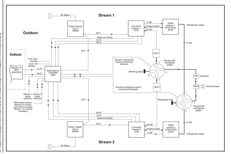
Figure power C-Band transceiver with separate RF waveguide switches Block diagram of the dual switch redundancy system for the low
