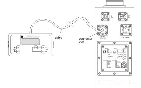
Figure 4-1: Connecting the controller to the converter
