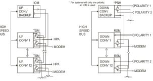
IOM=Input/Output Module TSM=Transit Switch Module RSM=Receive Switch Module PSM=Polarity Switch Module
