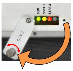
Figure 3-3. PCB-4000 LED Status Panel
