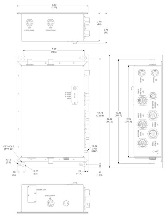
Figure 1-4. PCB-4300 Dimensional Envelope
