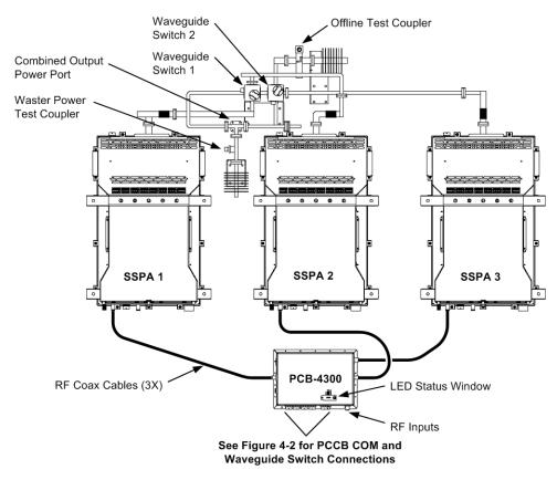
Figure 3-1. PCB-4300 1:2 Phase Combined System Assembly Example
