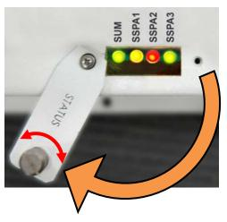
Figure 3-3. PCB-4300 LED Status Panel
