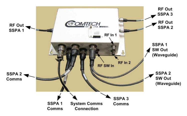
Figure A-10. Ku-Band 1:2 Phase Combined System Kit KT/11830-1 – PCCB Cabling Connections
