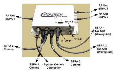
Figure 3-2. PCB-4300 1:2 Phase Combined System Cable Connections
