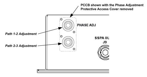
Figure 3-4. Phase Shifter Adjustment Locations
