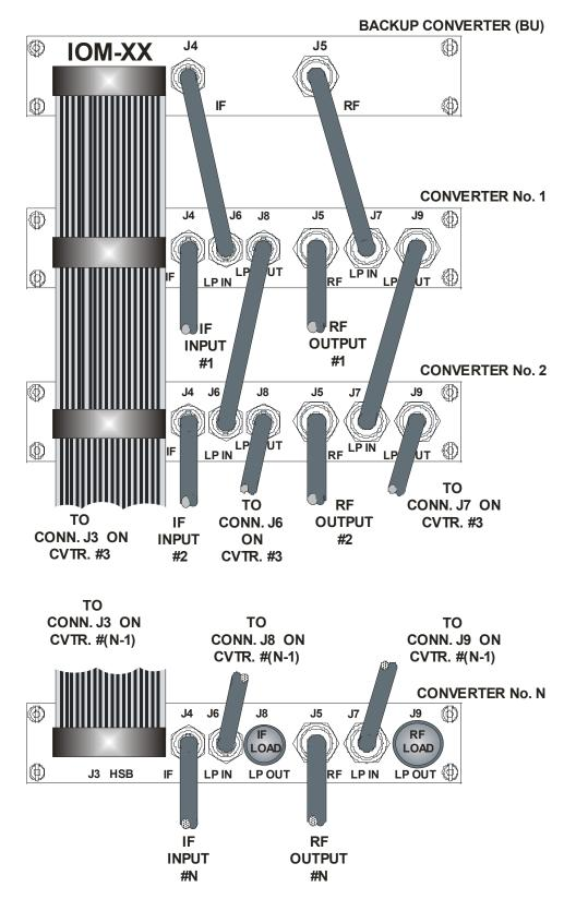
Figure 27. 1:N Redundant Configuration with IOM-XX and TSM-XX Installed
