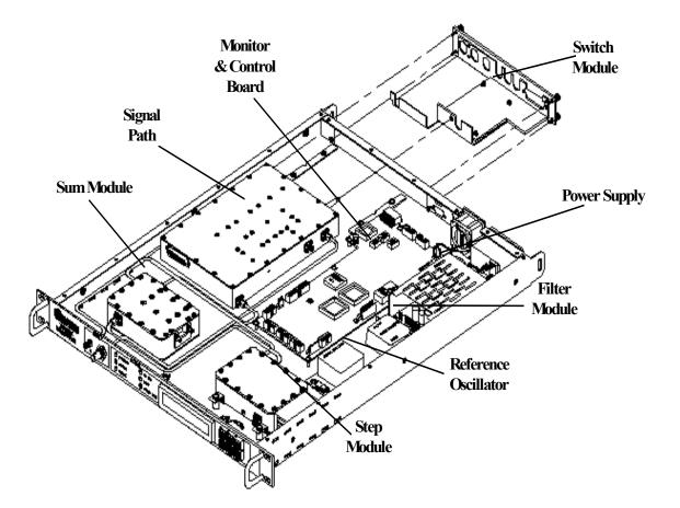
Figure 5. Physical Configuration - Up Converter
