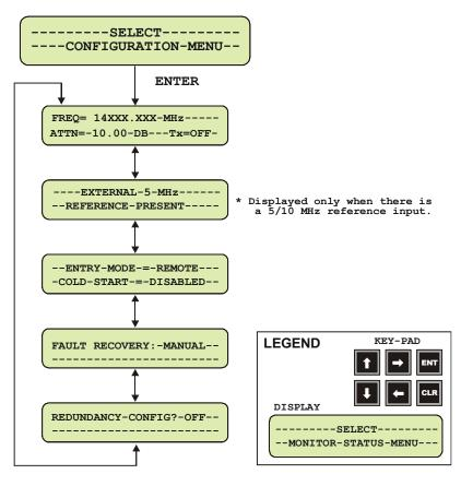
Figure 13. Configuration Menu Commands - Redundancy OFF.
