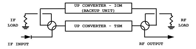
Figure 22. 1:1 Redundant Configuration Diagram - Single Source RF Input w/IOM-XX and TSM-XX Installed
