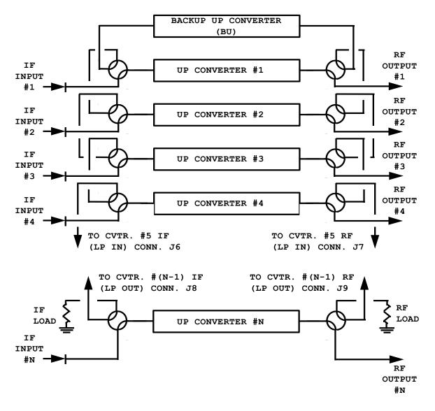
Figure 28. 1:N Redundant Configuration Diagram with IOM-XX and TSM-XX Installed
