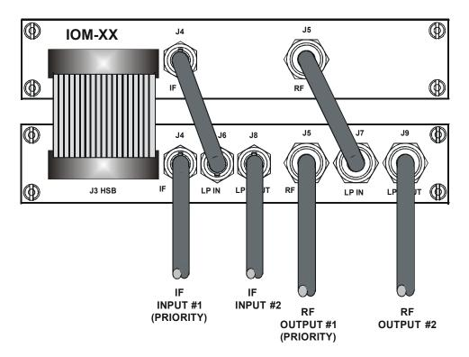
Figure 25. 1:1 Redundant Configuration - Dual Source IF Input
