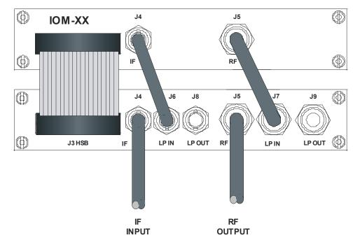
Figure 21. 1:1 Redundant Configuration - Single Source IF Input w/IOM and TSM-XX Installed
