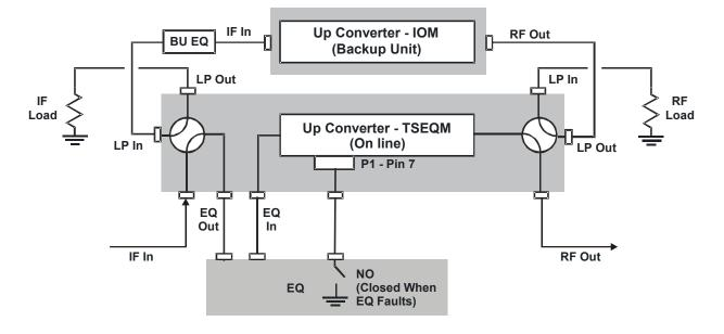
Figure 23. 1:1 Redundant Configuration Diagram -Single Source RF Input with IOM-XX and TSEQM-XX Installed
