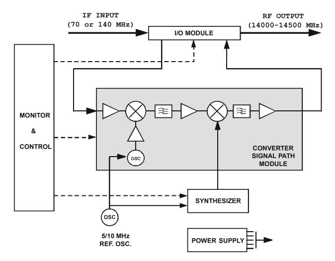
Figure 34. Typical Converter Functional Block Diagram (Model UT-4514 shown)
