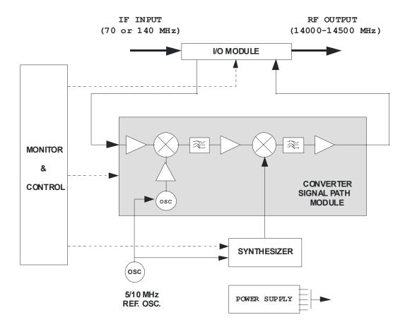
Figure 3. Typical Functional Block Diagram (Model UT-4514 shown)
