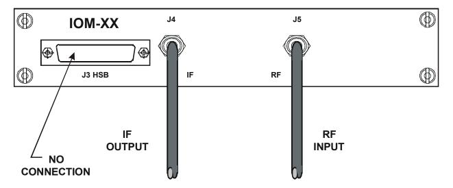
Figure 7. Non-Redundant Converter Configuration
