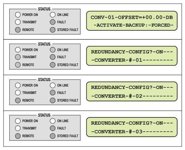
Figure 33. Forced BU of Converter #1
