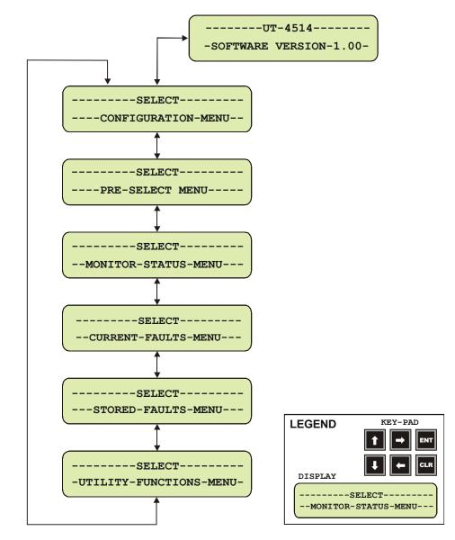
Figure 12. Converter Operating Command Functions
