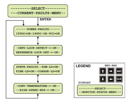
Figure 18. Current Faults Menu Commands
