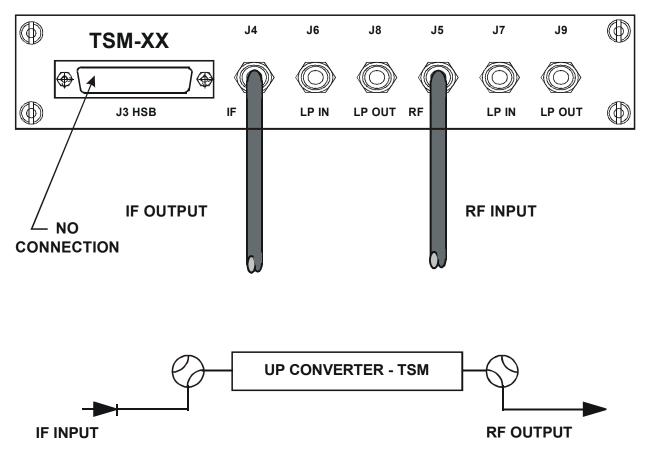
Figure 8. Non-Redundant Converter Configuration With Transmit Switch Module (TSM-XX) Installed
