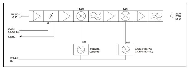
Figure 4-3. IF to S-Band Converter Module Block Diagram
