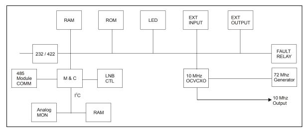
Figure 4-2. Monitor and Control (M&C) Block Diagram
