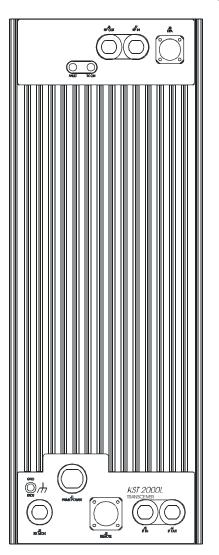
Figure 3-1. I/O View of KST-2000L Converter Unit
