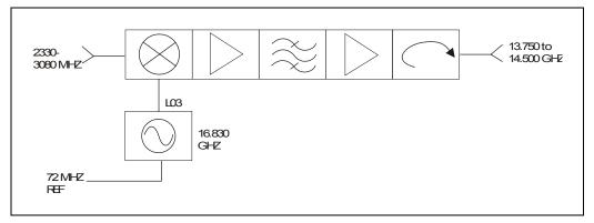
Figure 4-4. S to Ku-Band Up Converter Module
