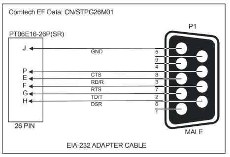
Figure 3-2. Serial (EIA-232) Adapter Cable Wiring Diagram
