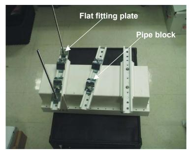
Figure 6-3. KST-2000L Converter with Mounting Brackets
