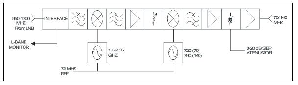
Figure 4-5. Ku-Band to IF Down Converter Block Diagram
