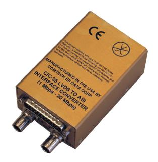
While the CDM-600/600L modem is capable of data rates up to 20 Mbps, its standard interface is limited to RS-422, V.35 and RS-232 and LVDS formats only. In order to accommodate the ASI format, a small converter box is available which attaches to the rear of the modem at the 25-pin data connector. No external power is required.
