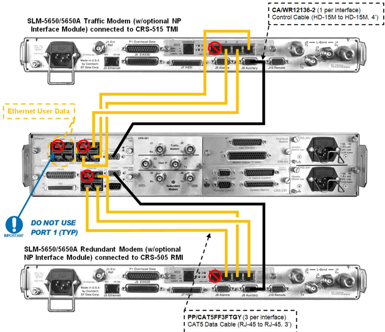
**Figure 3-12. SLM-5650/5650A Control and Ethernet Traffic (Multi-Port Bridge Mode) Data Cables**
