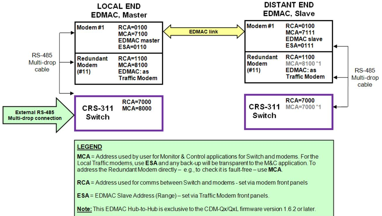
Figure B-5. CRS-311 Addressing Scheme Example: External RS-485 with CDM-Qx/QxL Modems, EDMAC CRS-311 to CRS-311
