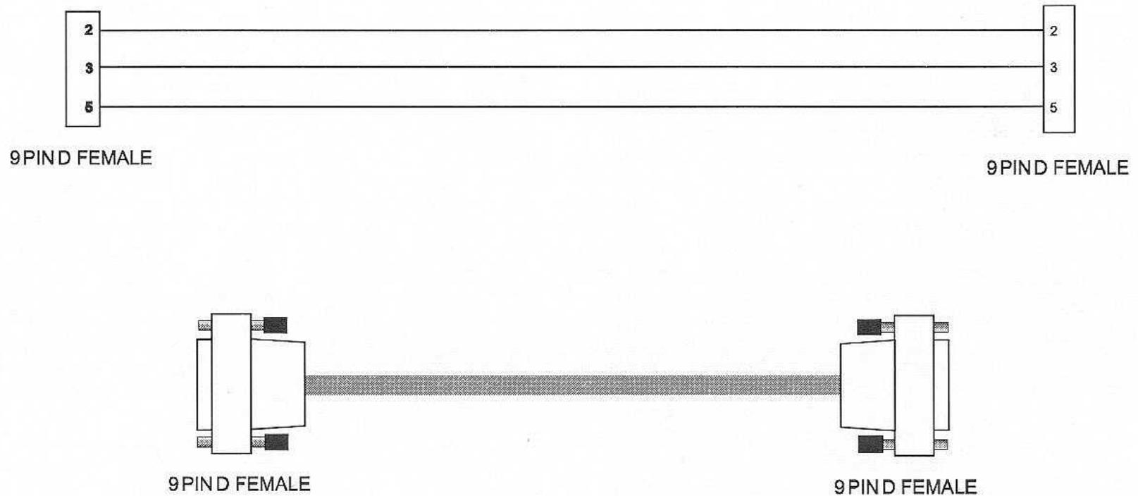
**Figure A-3. Switch Programming Cable**
