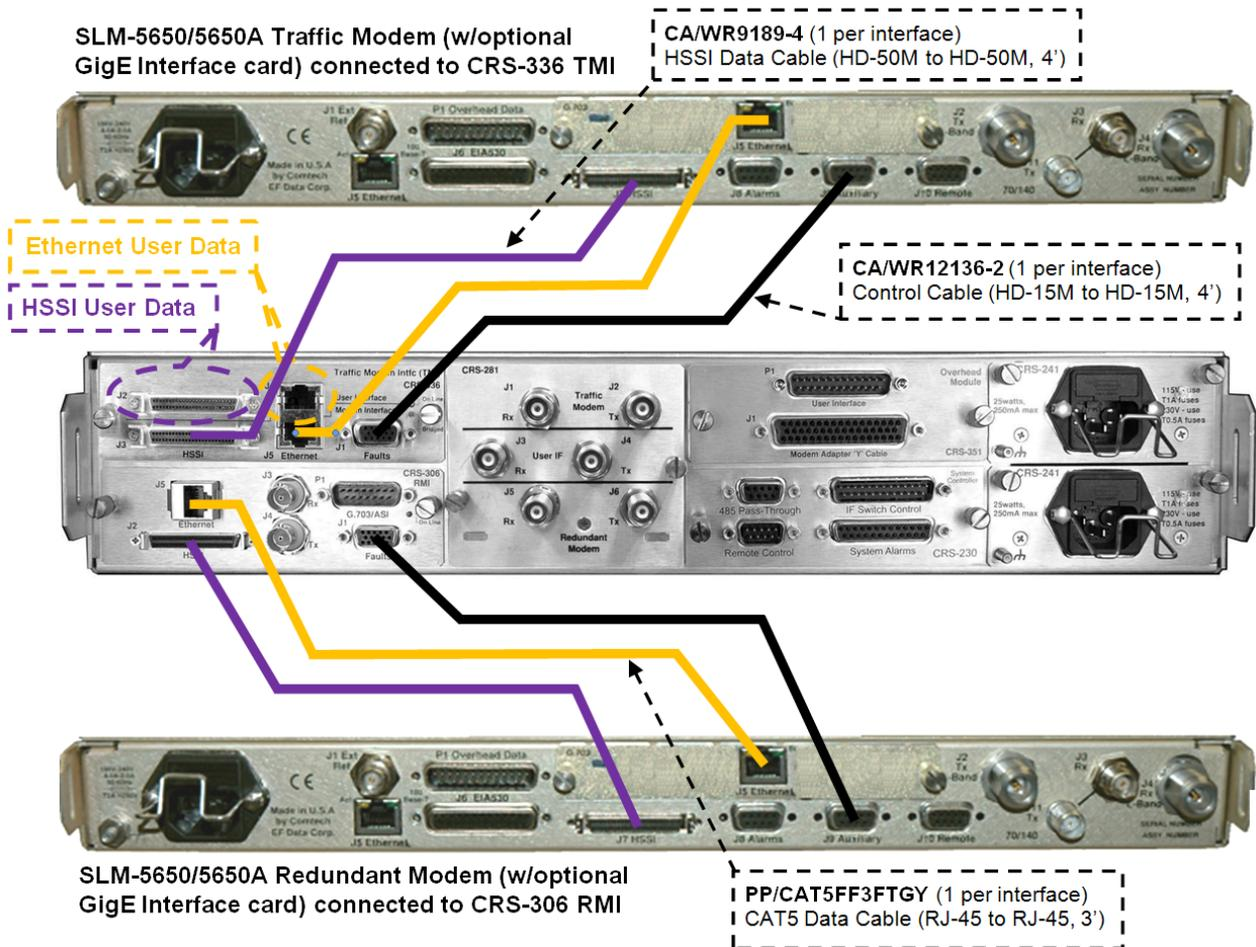
**Figure 3-9. SLM-5650/5650A Control and HSSI, Ethernet Traffic (Single Port Bridge Mode) Data Cables**
