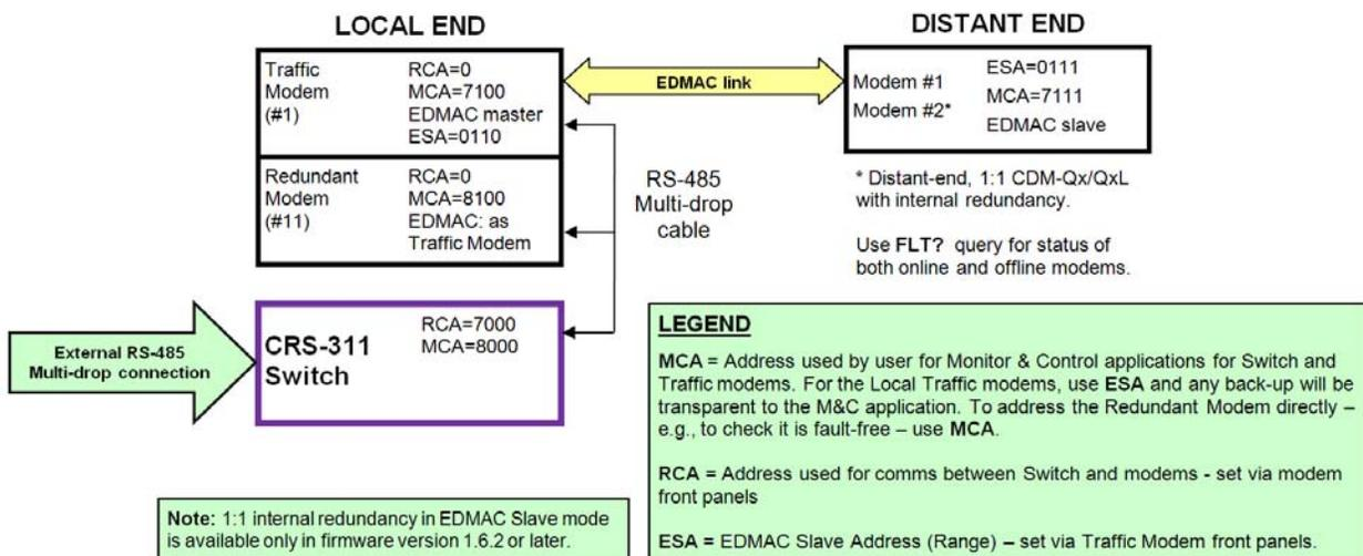
Figure B-4. CRS-311 Addressing Scheme Example: External RS-485 with CDM-Qx/QxL Modems
