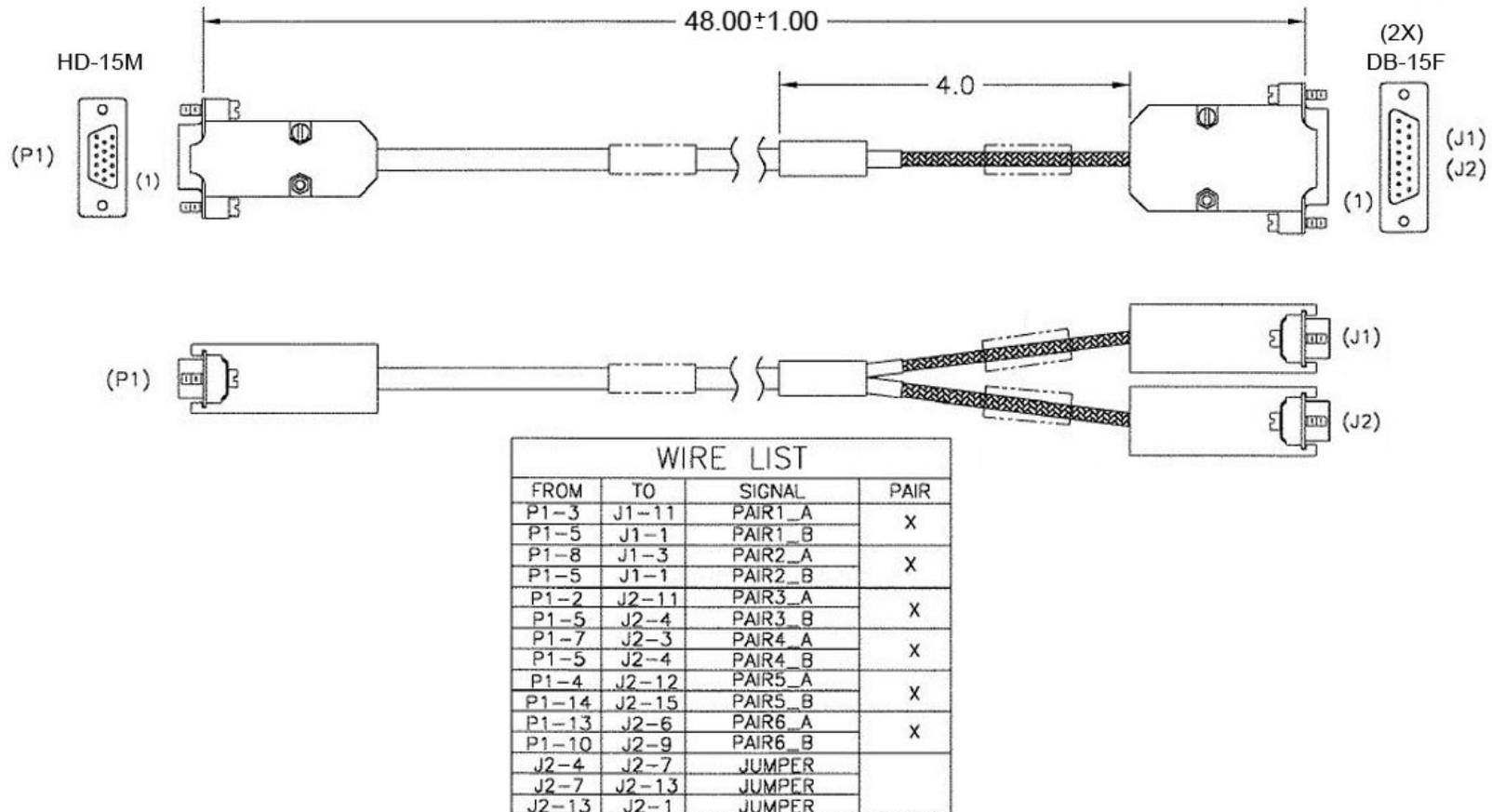
Figure A-8. Control 'Y' Cable for CDM-QxL with CnC® (CA-000009)
