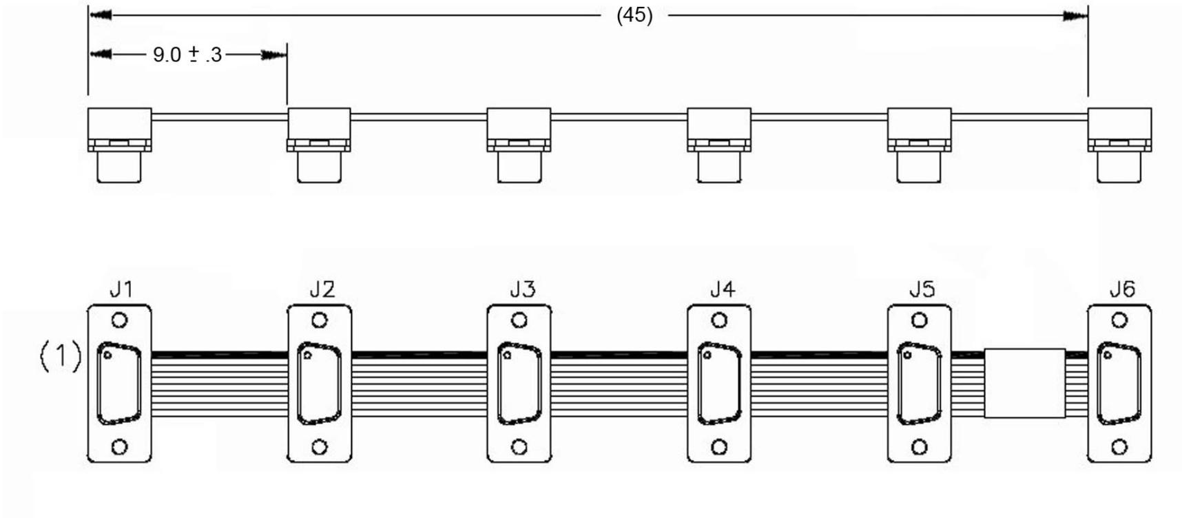
Figure A-4. Optional RS-485 Multi-Drop Ribbon Cable (CA-000095)
