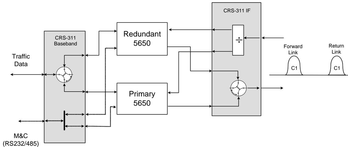
**Figure D-1. Standard Connections to CRS-311**
