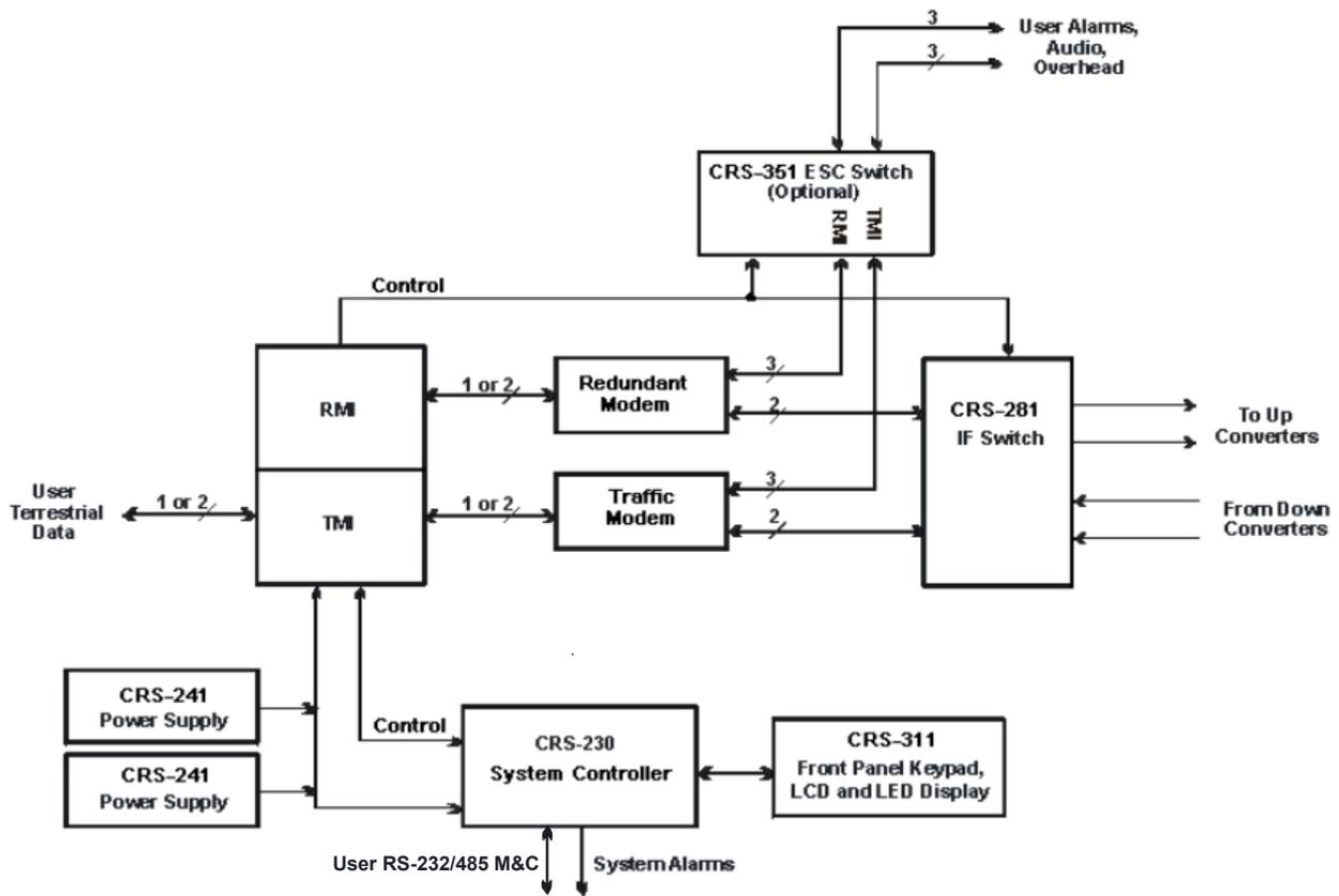
Figure 1-2. System-Level Block Diagram
