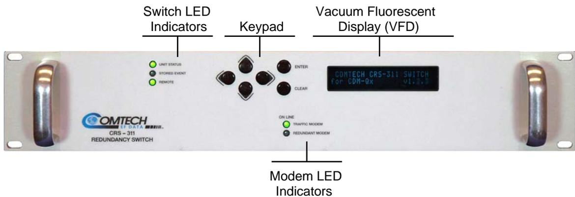
**Figure 6-1. CRS-311 Front Panel**
