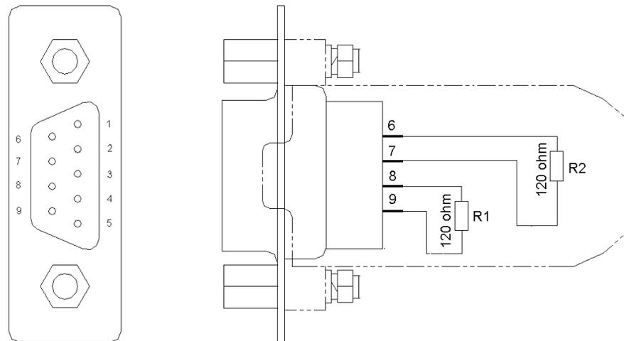
**Figure A-6. RS-485 Cable Termination (CA/WR11418-1)**
