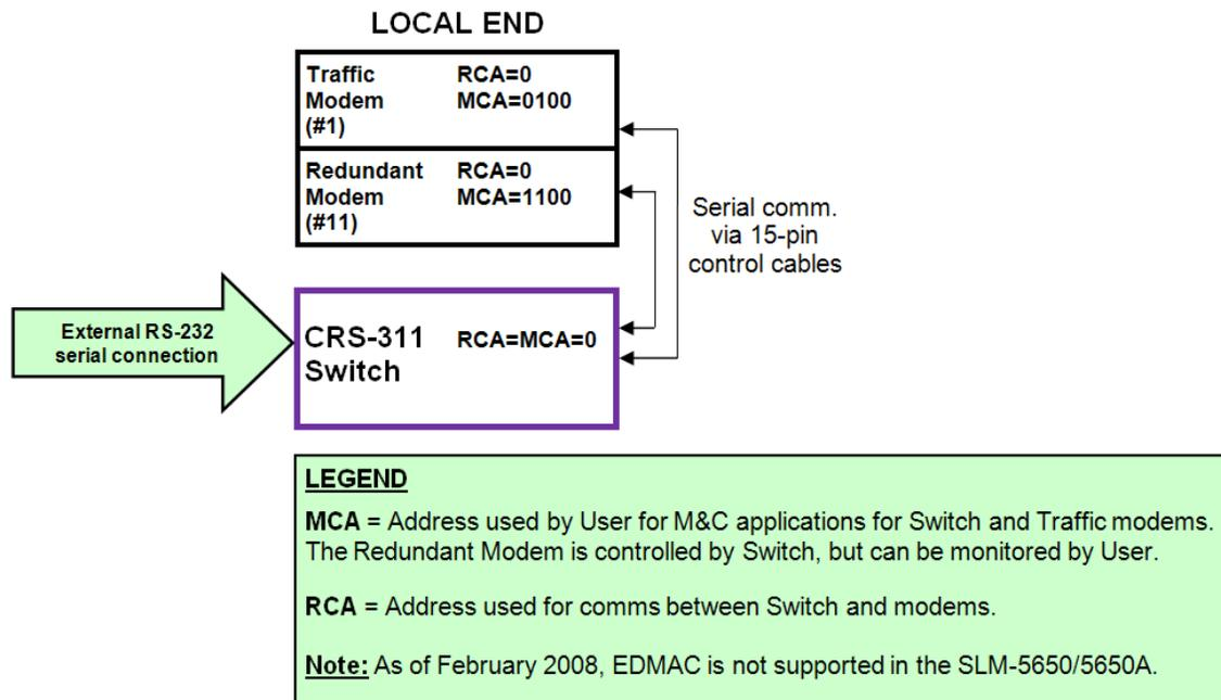
Figure B-1. CRS-311 Addressing Scheme Example: External RS-232 with SLM-5650/5650A Modems
