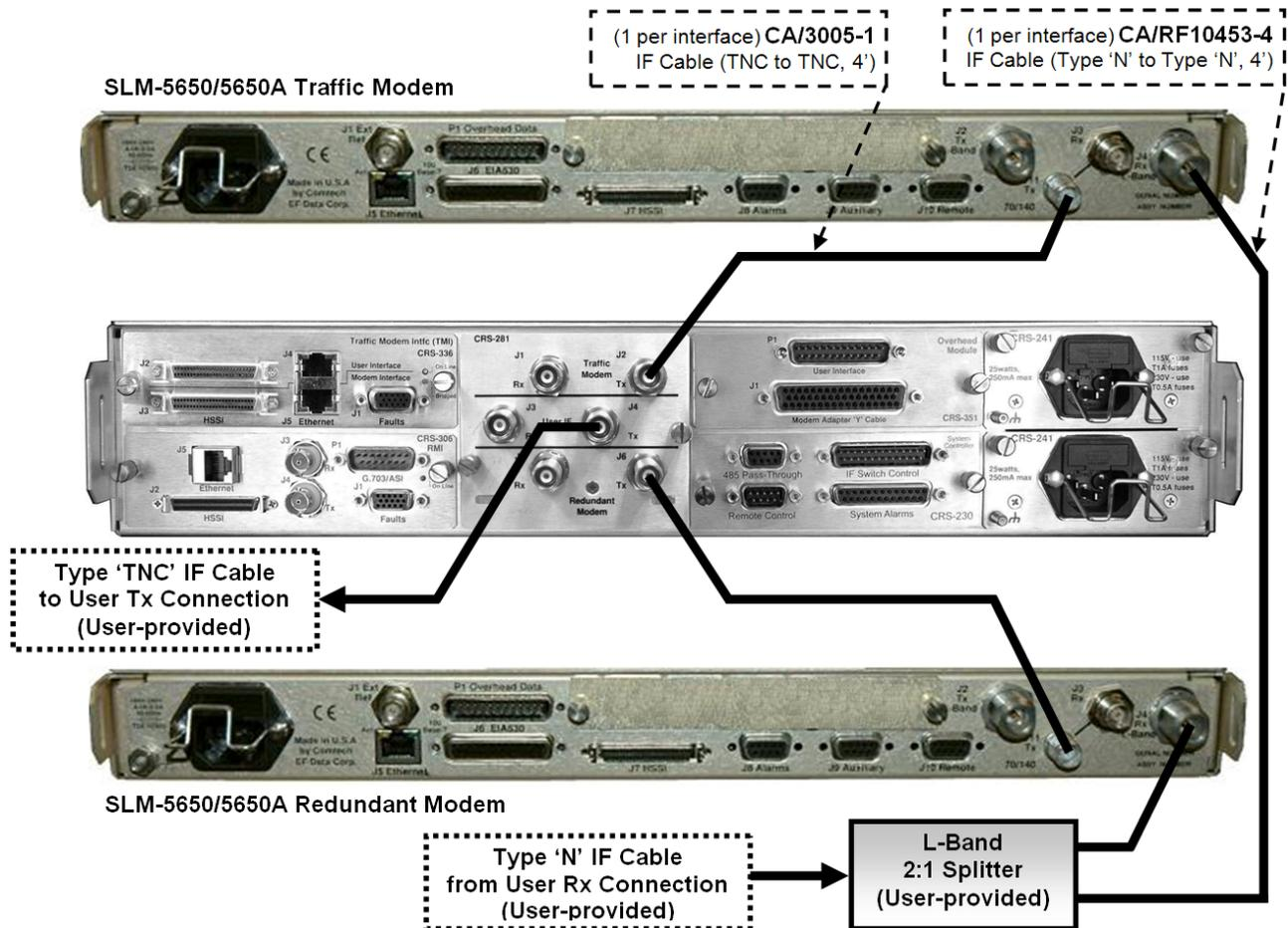
Figure 3-18. SLM-5650/5650A Mixed IF Band Cabling Example – CRS-281L (70/140 MHz Tx, L-Band Rx)
