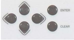
The keypad on the front panel contains six individual key switches with a positive “click” action for tactile feedback.
