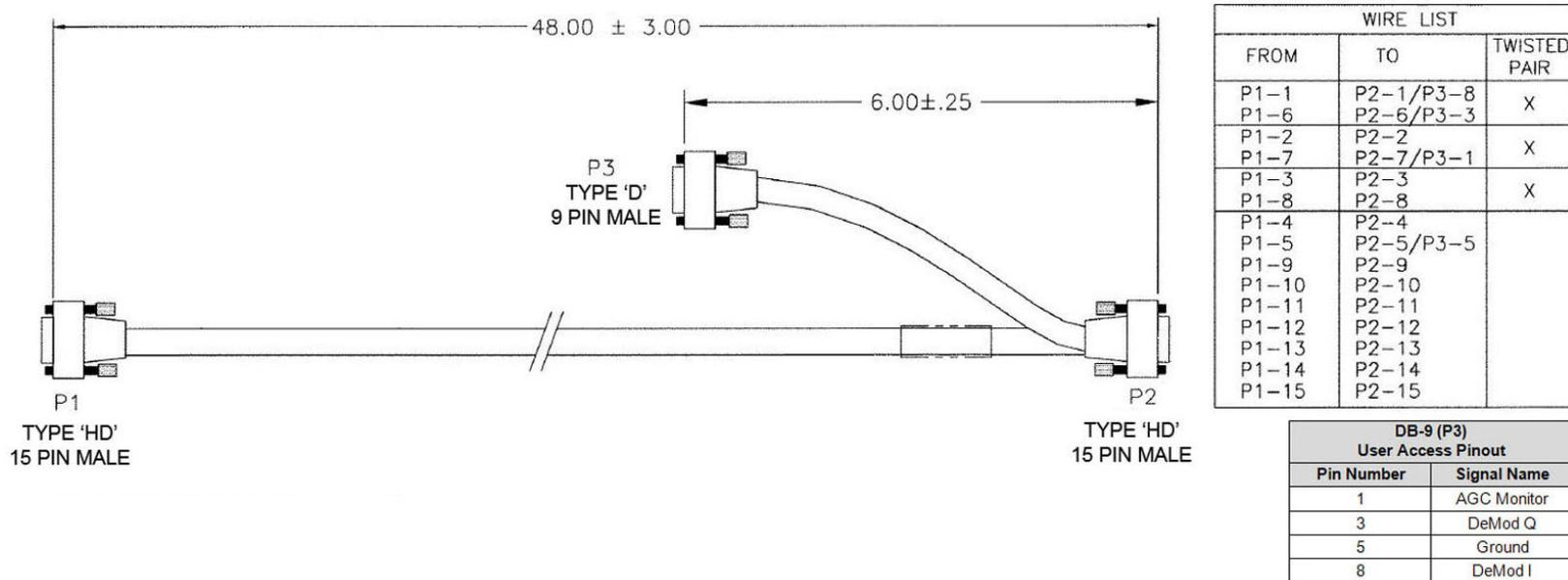
Figure A-11. SLM-5650/5650A Control 'Y' Cable (CA/WR12842-4)
