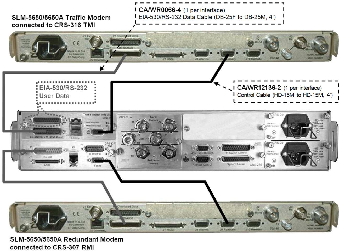
Figure 3-11. SLM-5650/5650A Control and EIA-530 Traffic Data Cables
