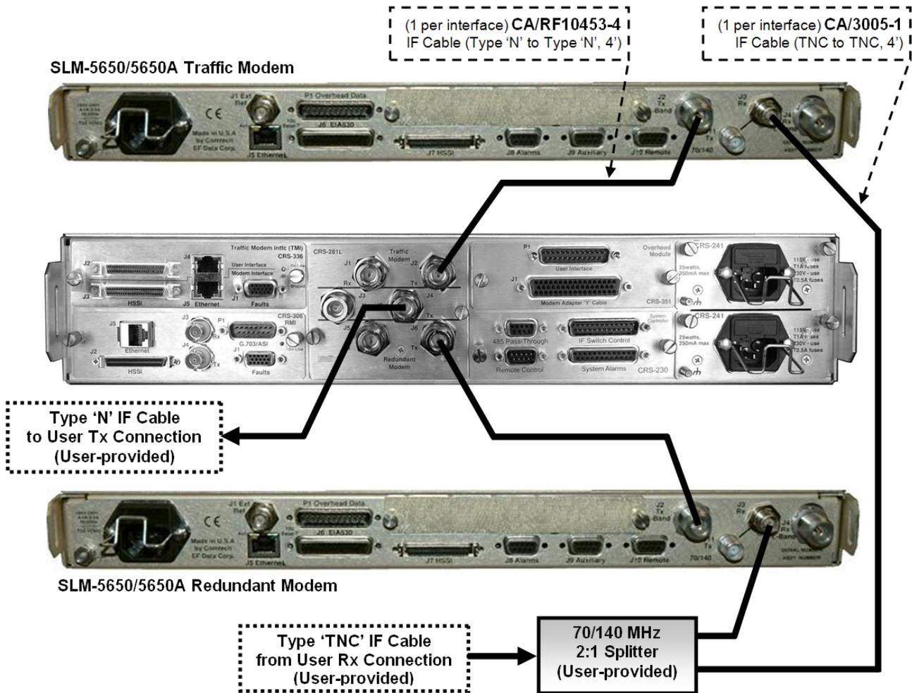
Figure 3-17. SLM-5650/5650A Mixed IF Band Cabling Example – CRS-281 'TNC' (70/140 MHz Tx, L-Band Rx)
