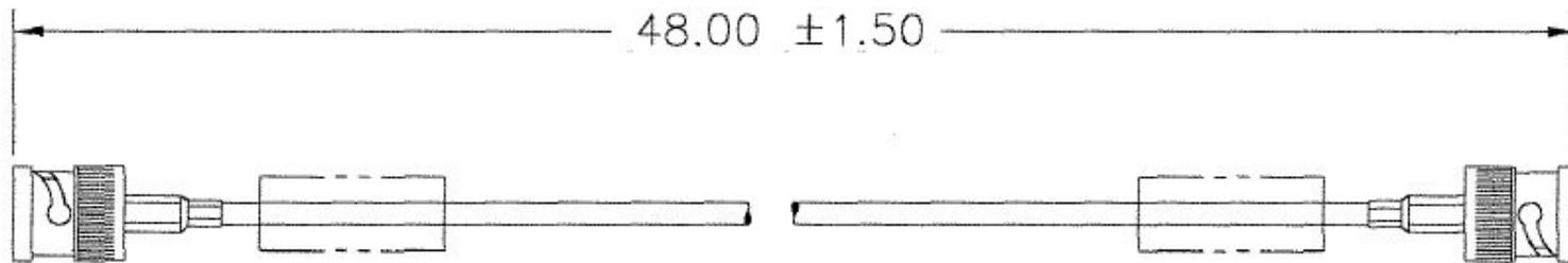
Figure A-14. Balanced G.703 / IF Cable, BNC 75Ω (PL/0813-4)
