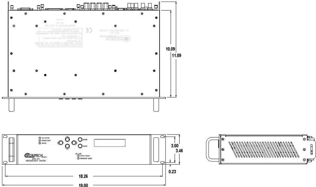
Figure 1-22. CRS-311 Dimensional Envelope
