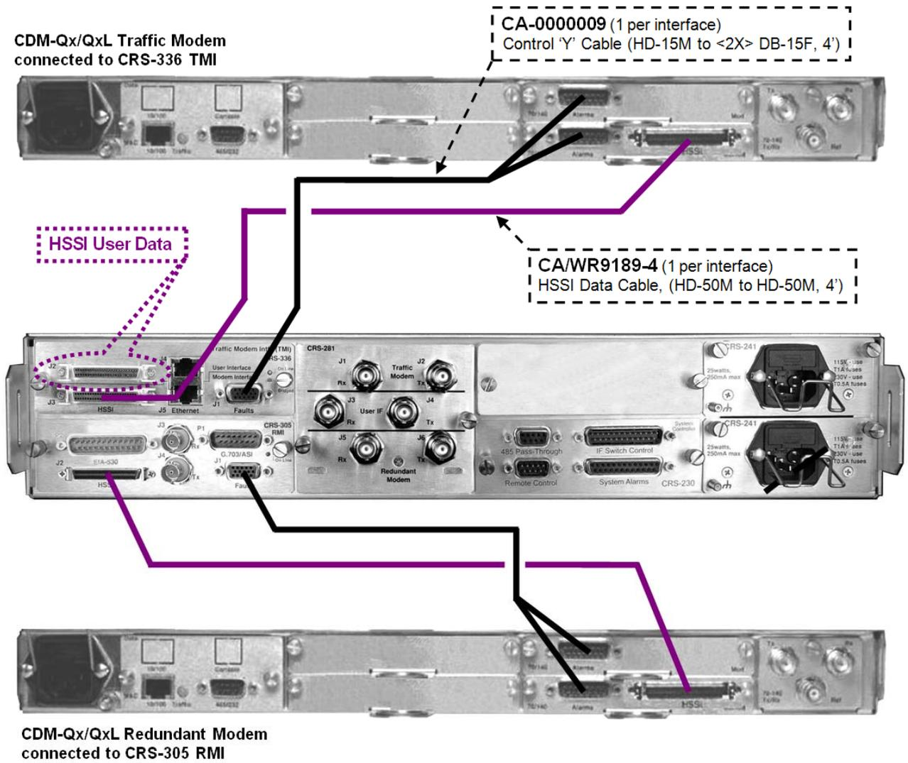
**Figure 3-5. CDM-Qx/QxL Control and HSSI Traffic Data Cables**
