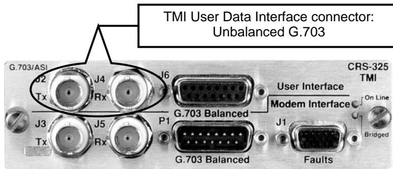
**Table 5-6** indicates the Unbalanced G.703 User Data Interface BNC connectors: “J2” and “J4” on the CRS-325 TMI.
