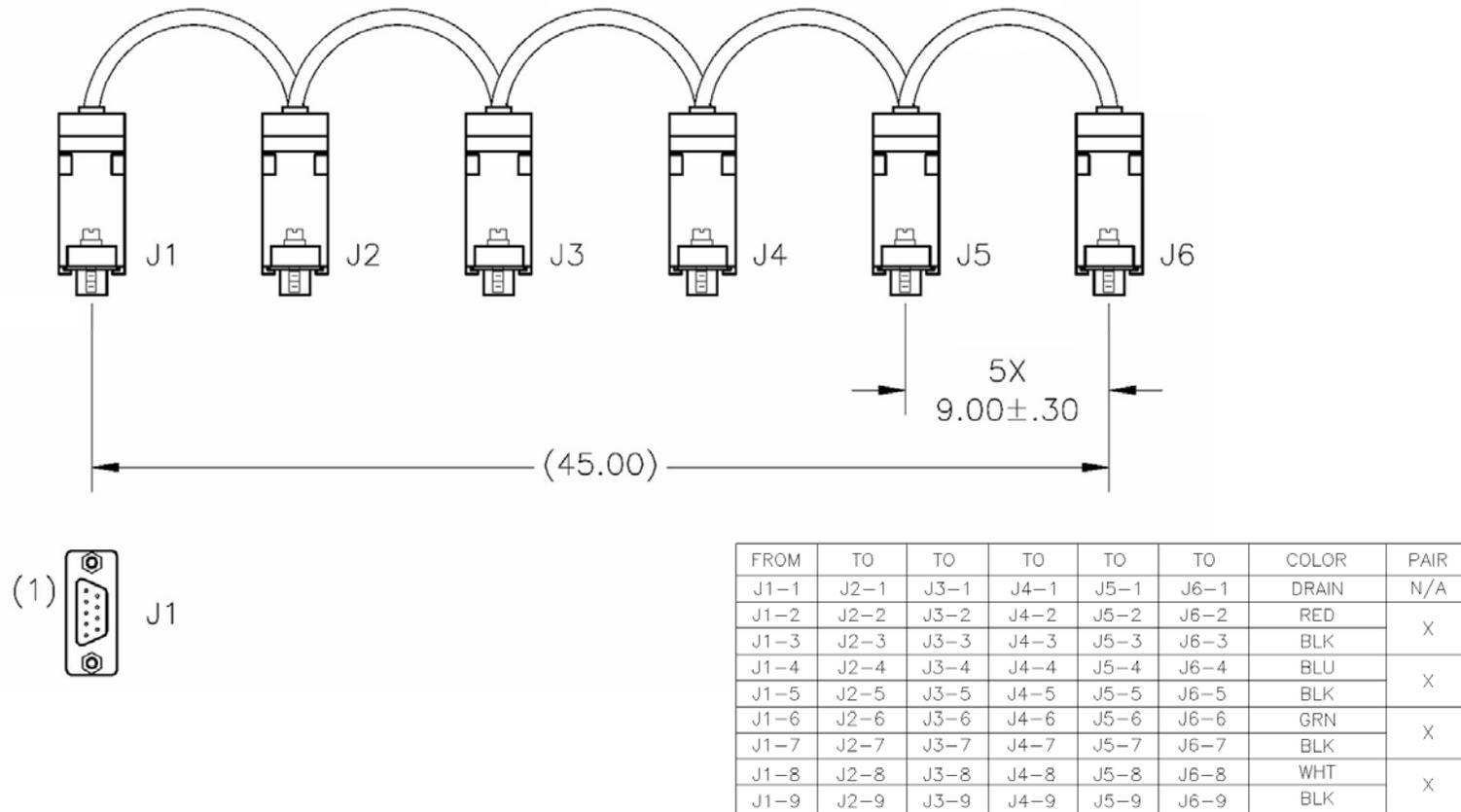
Figure A-5. Standard RS-485 Multi-Drop Shielded Cable (CA-000096)
