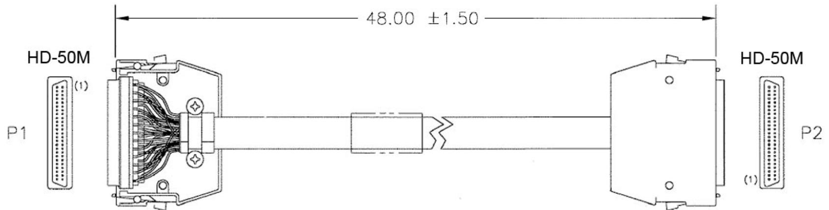
**Figure A-15. HSSI Data Cable (CA/WR9189-4)**
