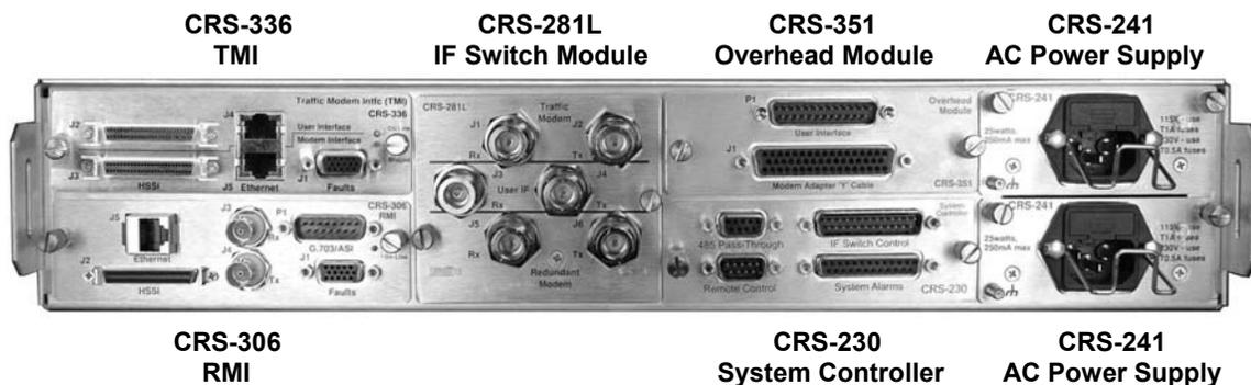
**Figure 1-4. CRS-311 Rear Panel Configuration Example**
