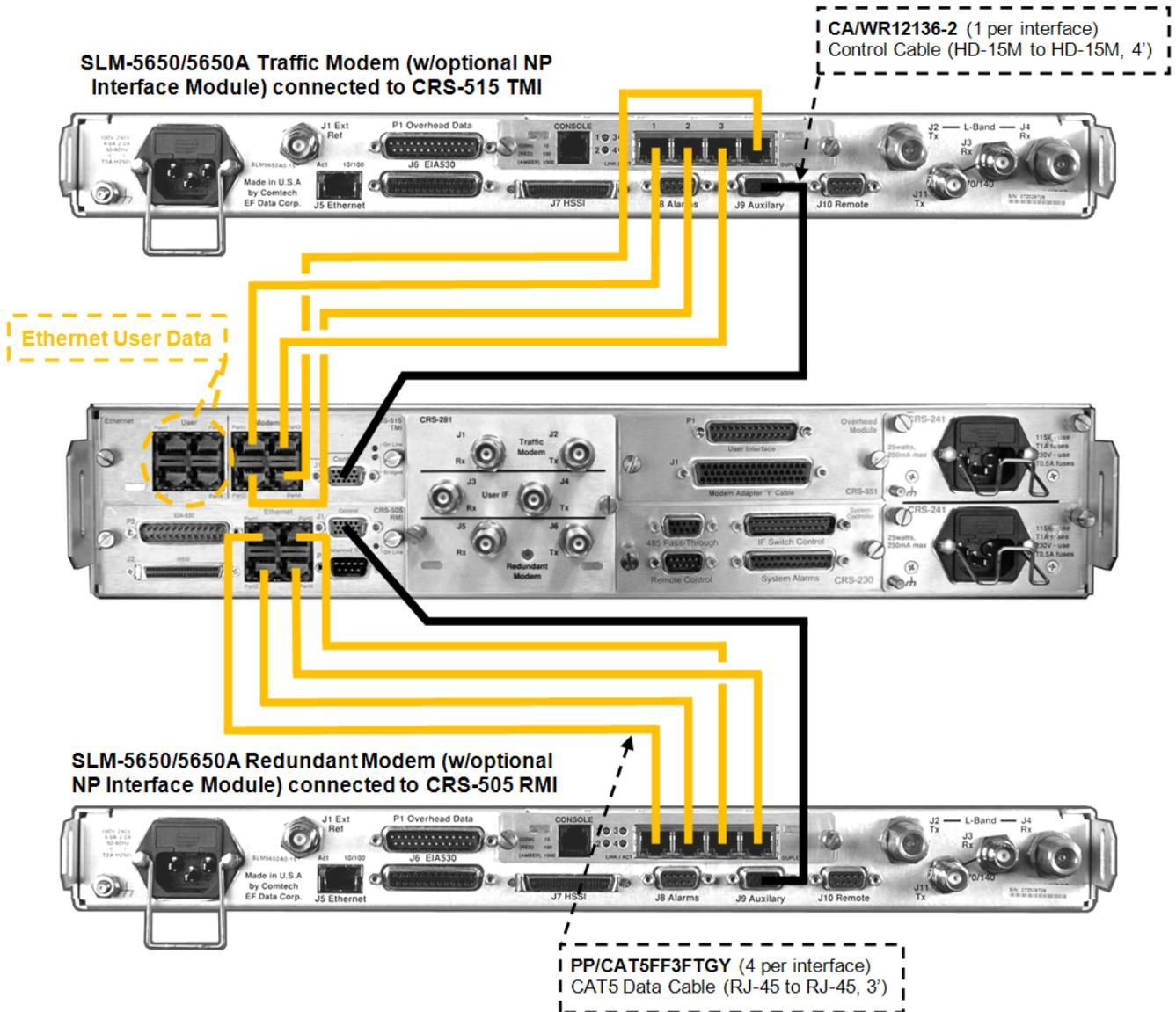
**Figure 3-13. SLM-5650/5650A Control and Ethernet Traffic (Multi-Port Router Mode) Data Cables**
