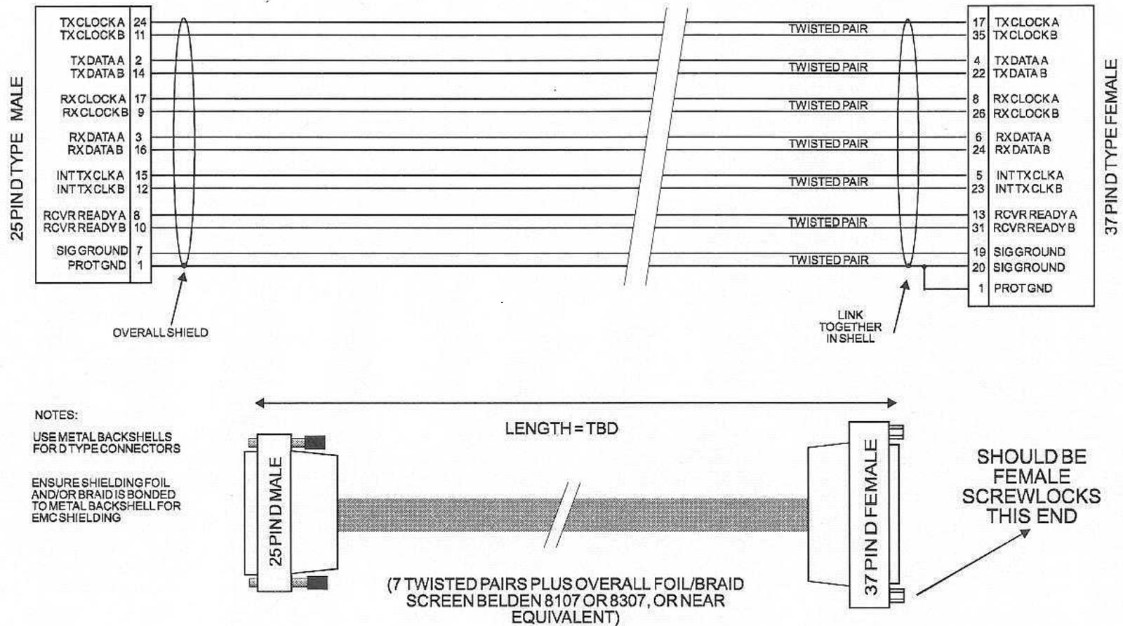
Figure A-1. DCE Conversion Cable: RS-530 to RS-422/449
