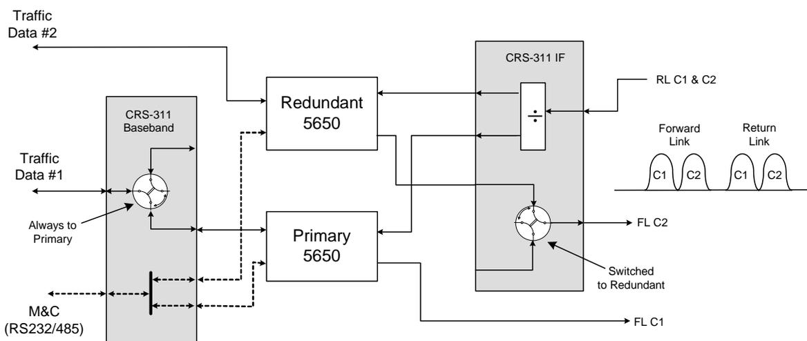
**Figure D-2: CRS-311 in Independent Mode**
