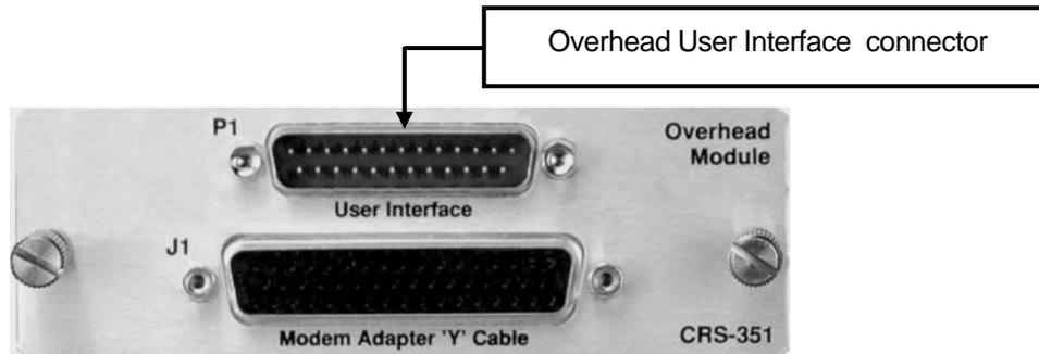
**Table 5-11** indicates pinout for the DB-25M Overhead User Data Interface connector: “P1” on the CRS-351 Overhead Module. This connector allows for connection of EIA-422, EIA-485 and EIA-232 data interfaces for use with overhead framing. It also supports signaling for tactical applications.
