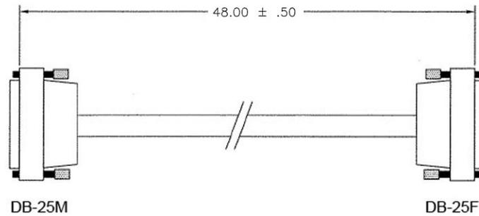
**Figure A-12. RS-232/422, EIA-530 Control and Data Cable (CA/WR0066-4)**
