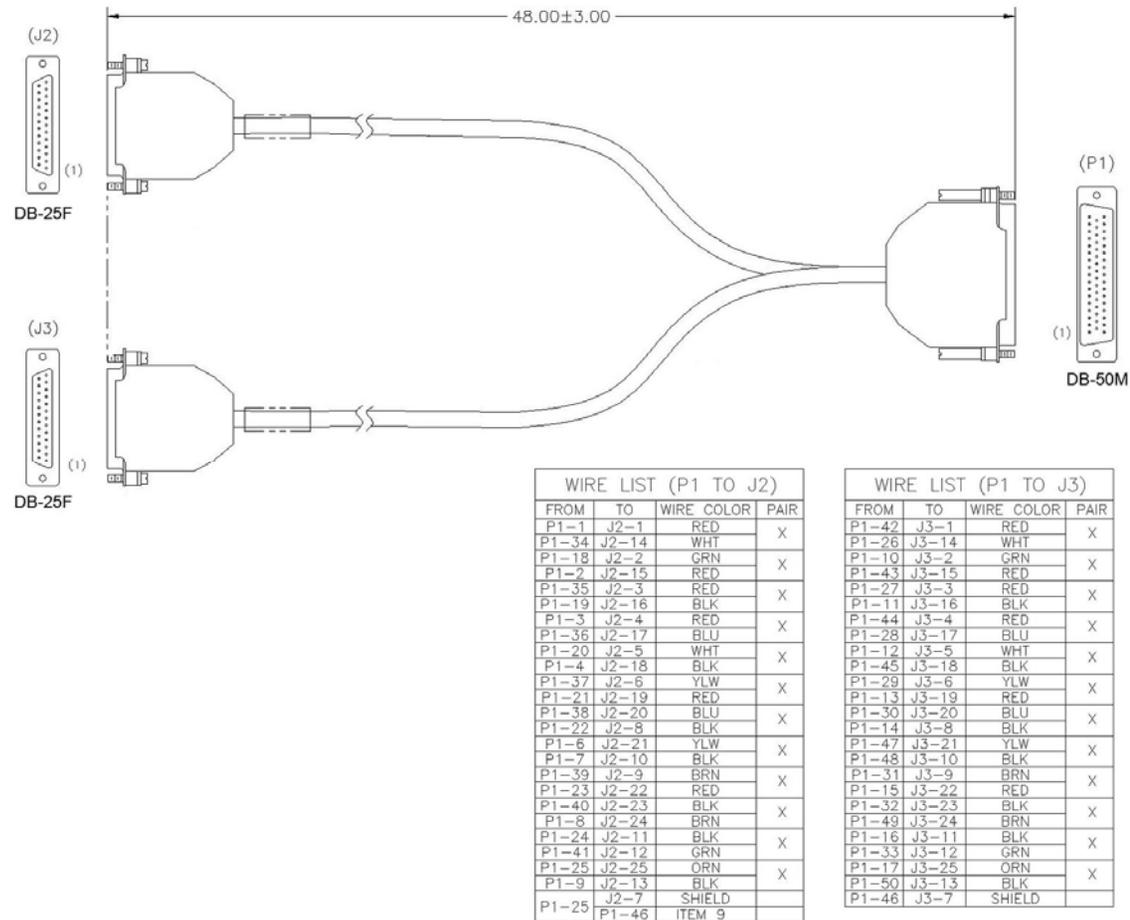
Figure A-10. SLM-5650/5650A Control 'Y' Overhead Cable (CA-000006)
