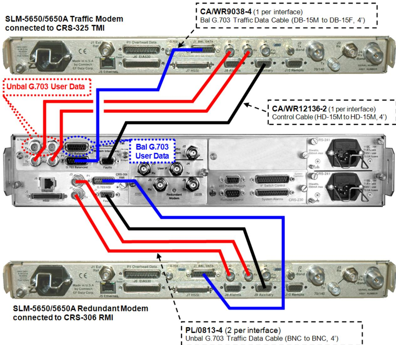
Figure 3-10. SLM-5650/5650A Control and G.703 Traffic Data Cables
