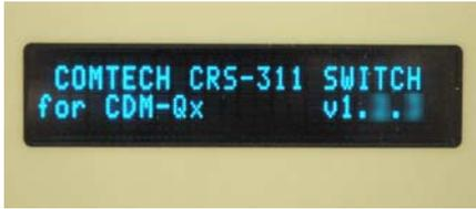
This screen is displayed whenever power is first applied to the unit. The display has two lines each of 24 characters. The second line identifies the modem for which the CRS-311 is configured (e.g., SLM-5650, CDM-Qx, etc.), and the CRS-311's installed firmware version.
