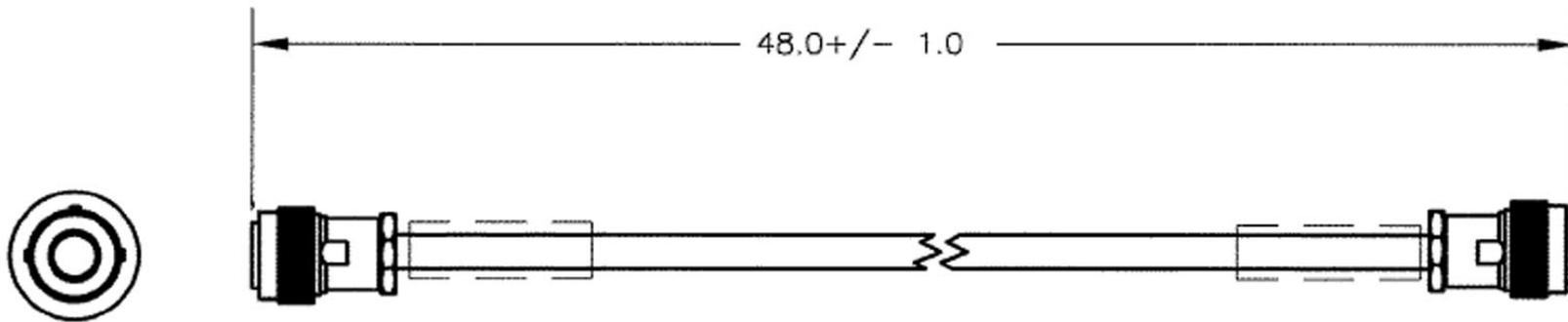
Figure A-20. IF Cable, TNC 50Ω for CRS-281 (70/140 MHz) IF Switch (CA/3005-1)
