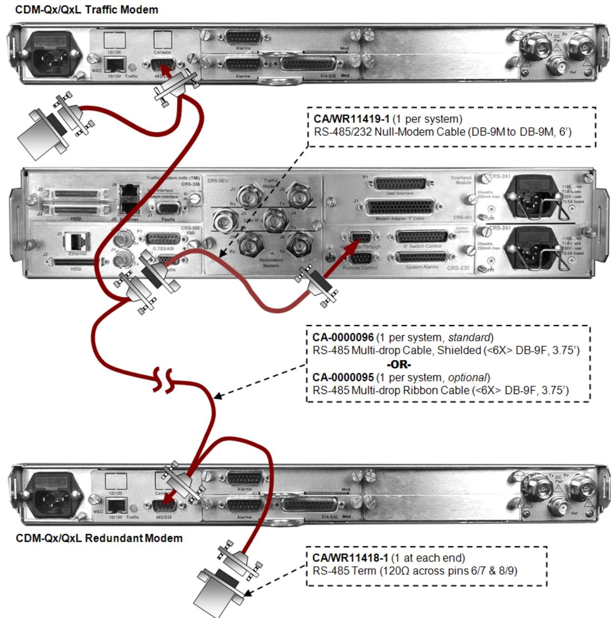
**Figure 3-1. CDM-Qx/QxL Cabling Example – RS-485 Multi-drop Cable**
