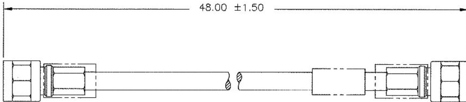
**Figure A-19. IF Cable, Type 'N' 50Ω for CRS-281A / CRS-281L (L-Band) IF Switches (CA/RF10453-4)**
