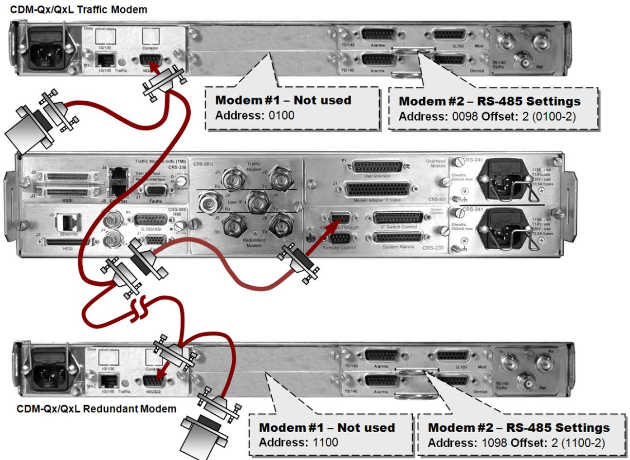
**Figure 4-2. CDM-Qx/QxL / CRS-311 RS-485 Scheme**
