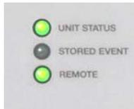
The three LEDs positioned at the top left of the front panel reflect the condition of the Switch itself. The function of these LEDs is as follows:
