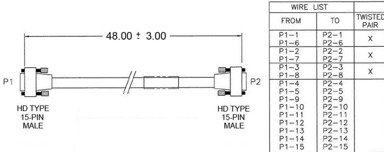
Figure A-9. SLM-5650/5650A Control Cable (CA/WR12136-2)
