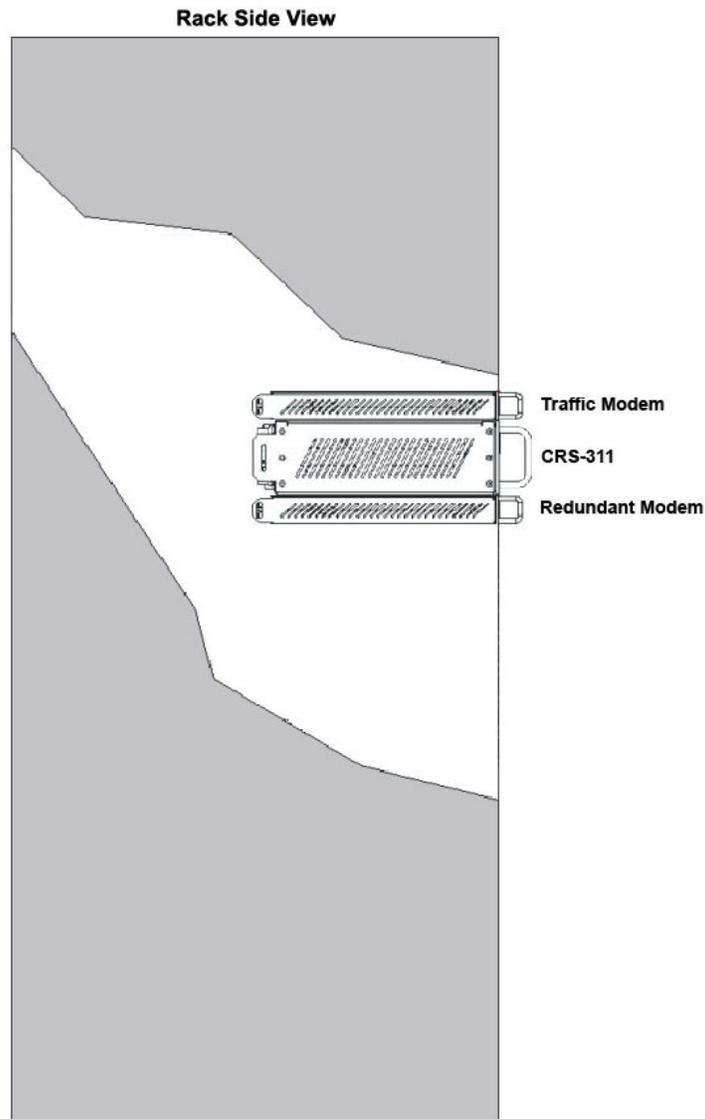
**Figure 2-1. Typical Rack-mounted Configuration**
