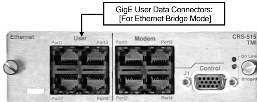
**Table 5-10** indicates the pinout for the RJ-45F TMI User Data Interface connectors Gigabit Ethernet (GigE) connectors: “Port1” through “Port4” on the CRS-515 TMI.
