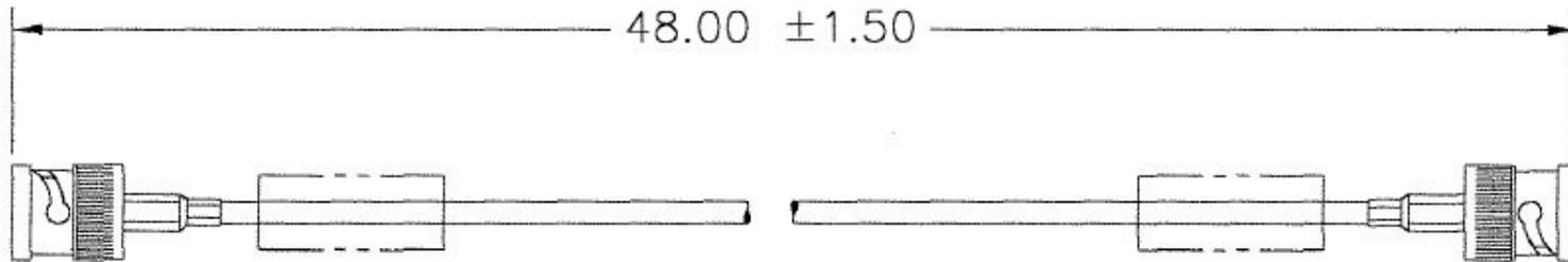
**Figure A-18. IF Cable, BNC 50Ω for CRS-281 (70/140 MHz) IF Switch (PL/0946-1)**
