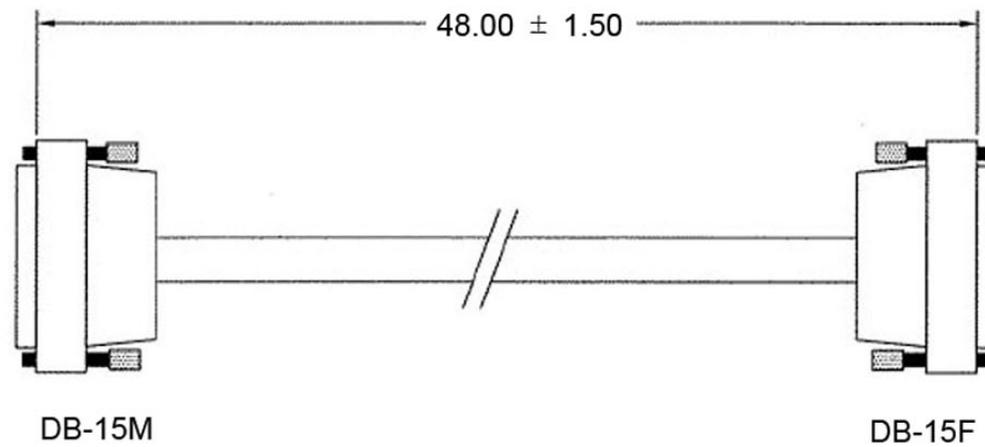
Figure A-13. Balanced G.703 Data Cable (CA/WR9038-4)
