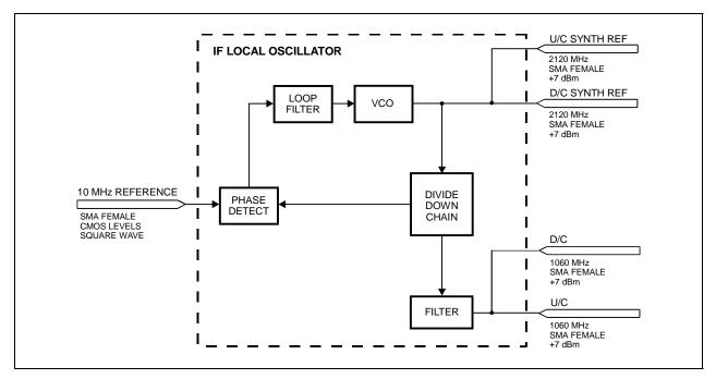
Figure 6-5. IF Local Oscillator Block Diagram
