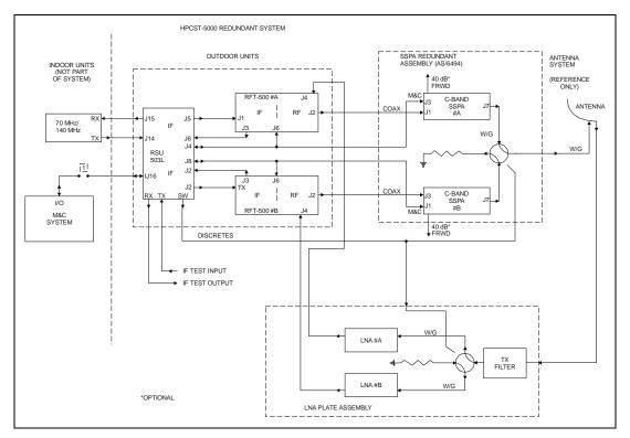
Figure 4-1. HPCST-5000 Redundant System Schematic Using SSPAs
