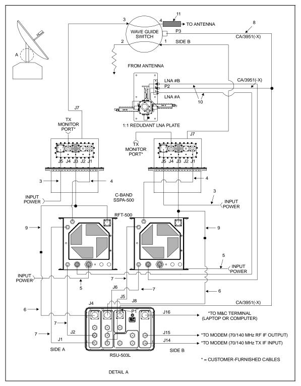
Figure 8-2. 1:1 Redundant Configuration Cabling
