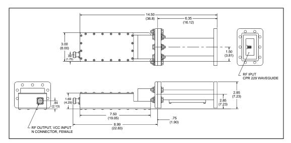
**Figure 1-9. Single Thread Configuration Dimensional Requirements**
