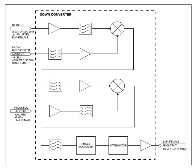
Figure 6-8. Down Converter Block Diagram
