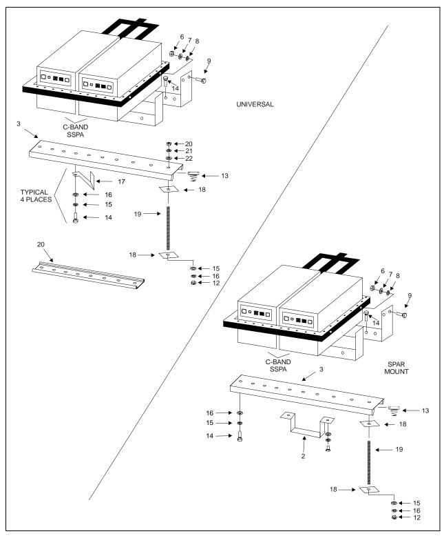
Figure 8-6. 1:1 Redundant System Universal Mounting Kit (KT/6700)
