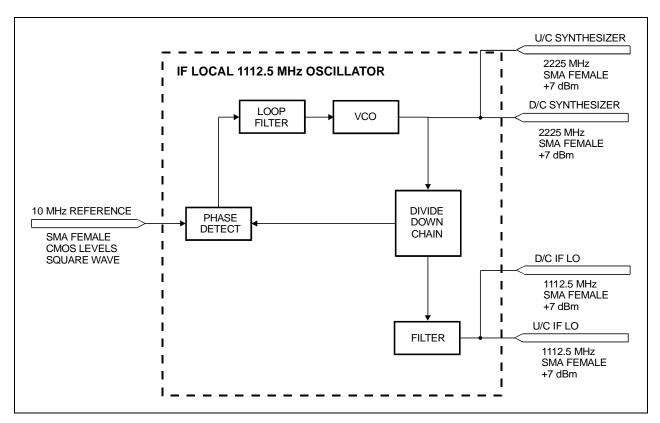
Figure A-1. IF Local Oscillator Block Diagram
