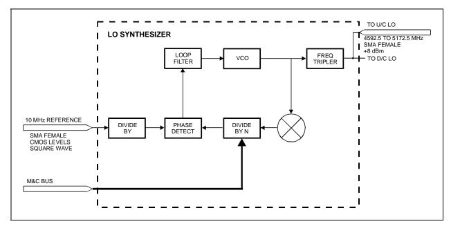
Figure A-3. U/C LO Synthesizer Block Diagram
