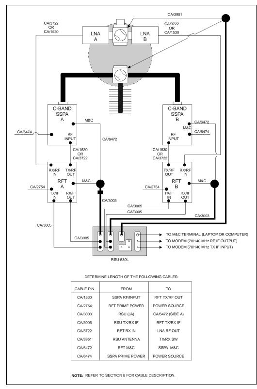
Figure 4-5. Redundant Configuration Cable Assembly Matrix
