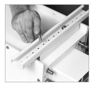
**Note:** The bolts should be installed in the fifth hole from each end, as illustrated.
