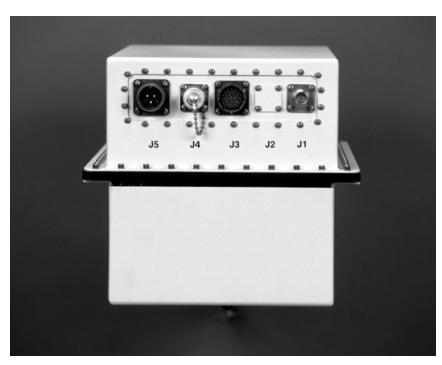
Figure 2-3. C-Band SSPA External Connections
