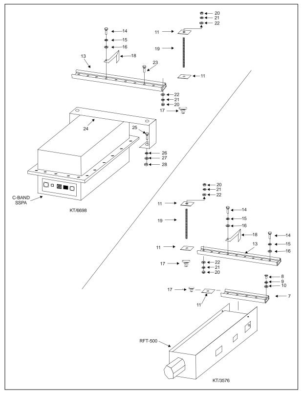
Figure 8-4. Exploded View of Universal Mounting Kit
