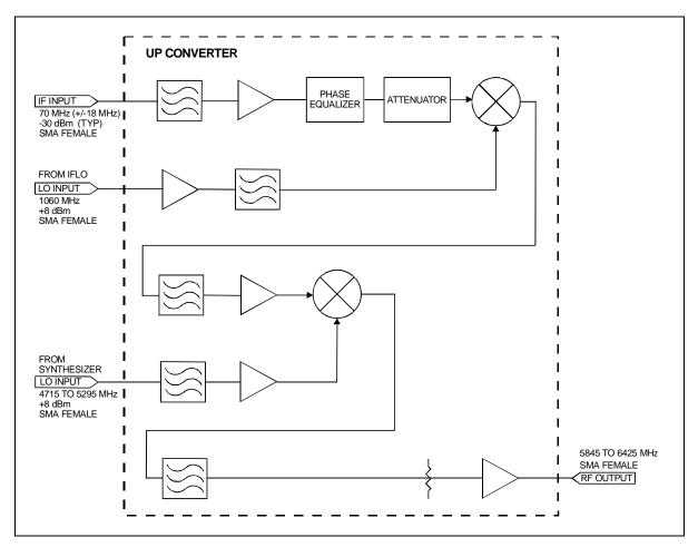
Figure 6-9. Up Converter Block Diagram
