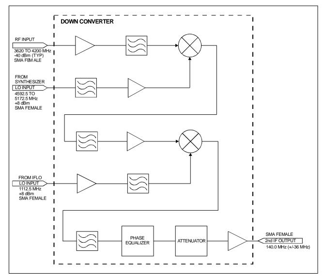
Figure A-4. Down Converter Block Diagram
