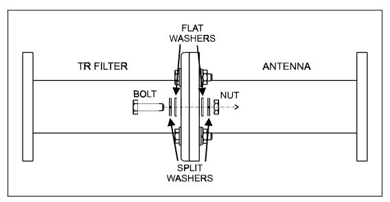
Figure 4-3. Installation of LNA to Waveguide
