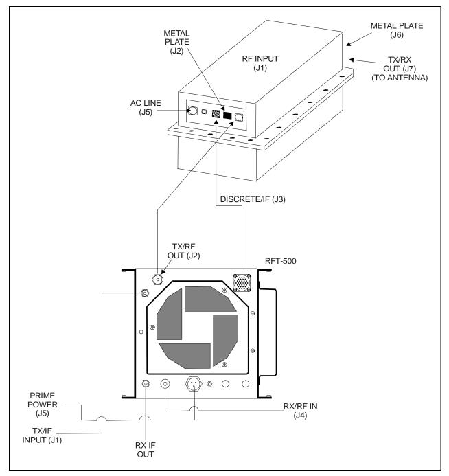
Figure 3-1. HPCST-5000 Single Thread Configuration Schematic
