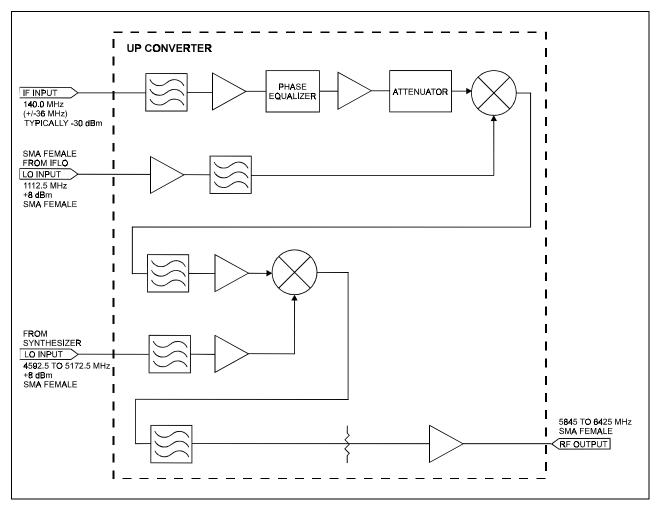
Figure A-5. Up Converter Block Diagram
