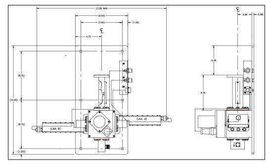
Figure 1-10. Standard Redundant Configuration Dimensional Requirements
