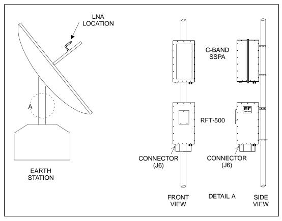
Figure 1-3. Typical View of Single Thread Installations
