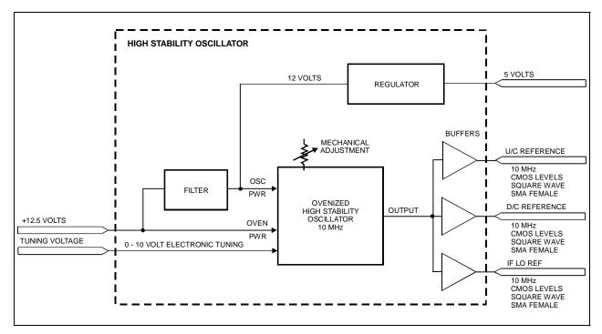
Figure 6-4. High Stability Oscillator Block Diagram
