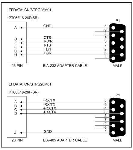
Figure 2-2. Serial Adapter Cables
