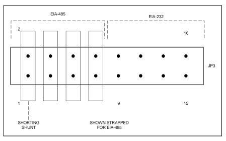
Figure 6-2. M&C Jumper Placement at JP3
