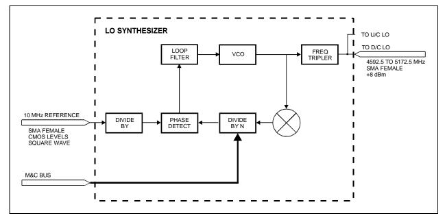
Figure A-2. LO Synthesizer Block Diagram
