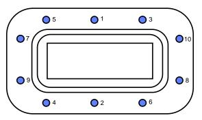
Figure 4-4. Procedures for Tightening LNA to Waveguide Bolts
