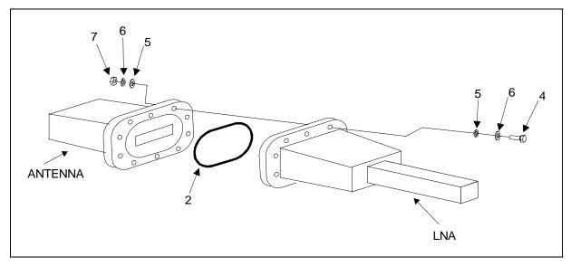
Figure 8-1. Exploded View of a Typical LNA Connector Kit
