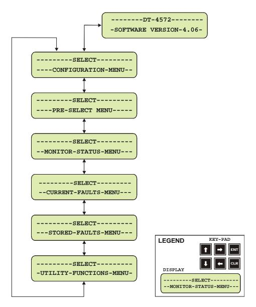
Figure 12. Converter Operating Command Functions
