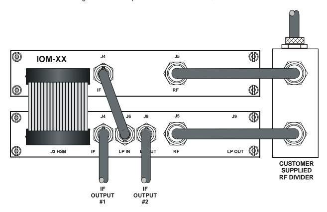
Figure 24. 1:1 Redundant Configuration - Dual Source IF Input
