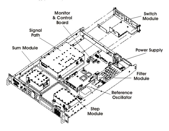
Figure 5. Physical Configuration - Down Converter
