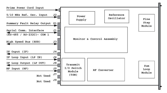
Figure 6. Converter Signal and Interconnecting Cable Diagram (with TSM Switching Module)
