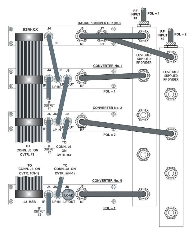
Figure 26. Dual Source1:N Redundant Configuration with PSM-XX and RSM-XX Installed
