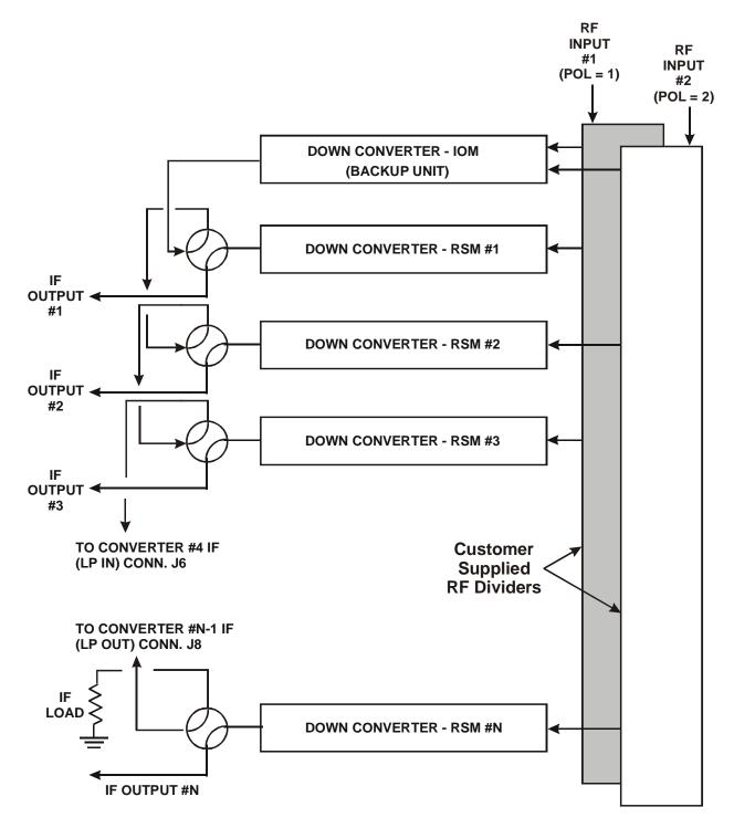
Figure 27. Dual Source 1:N Redundant Configuration Diagram with PSM-XX and RSM-XX Installed
