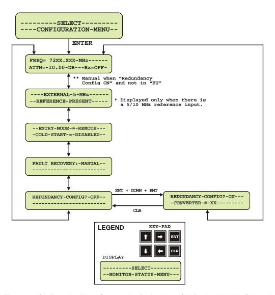
Figure 14. Configuration Menu Commands - Redundancy ON, Backup Unit Not Selected
