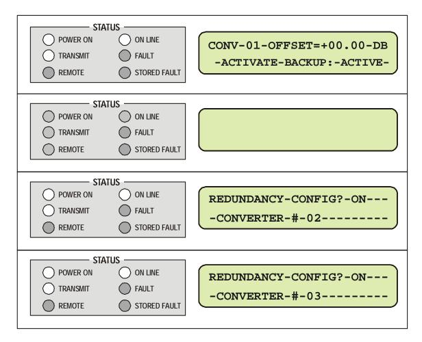
Figure 30. Converter #1 Being Backed Up
