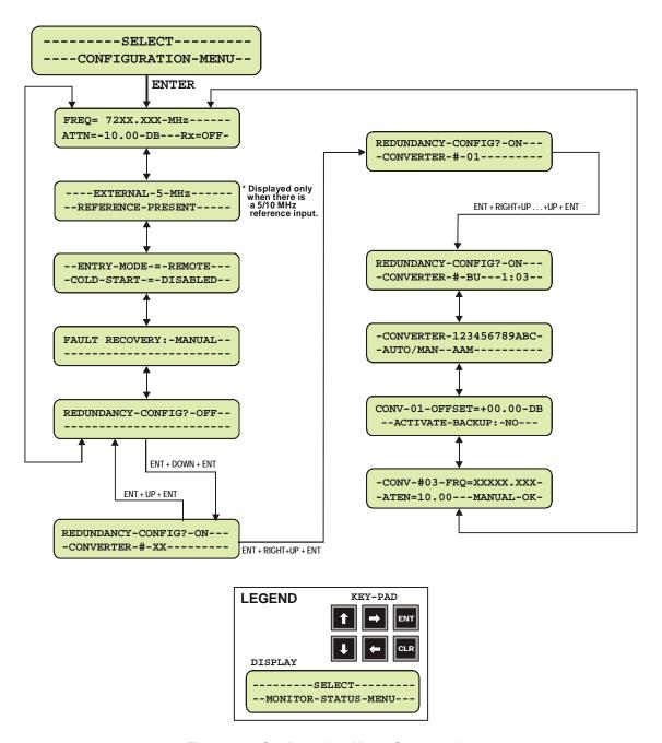
Figure 15. Configuration Menu Commands - Redundancy ON and Backup Unit Selected
