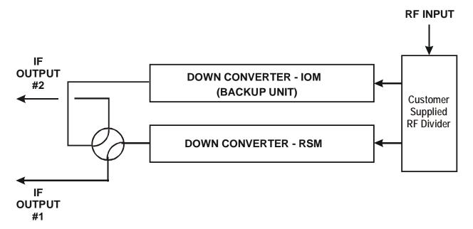
Figure 25 1:1 Redundant Configuration Diagram Dual Source IF Output with IOM-XX and RSM-XX Installed.
