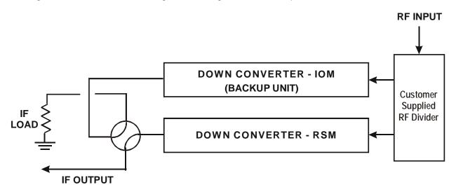
Figure 22. 1:1 Redundant Configuration Diagram - Single Source IF Output w/IOM and RSM-XX Installed
