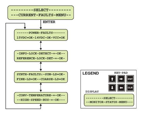
Figure 18. Current Faults Menu Commands
