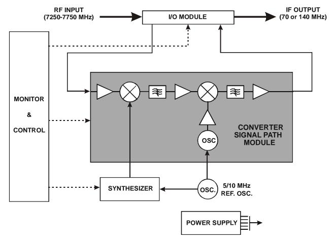
Figure 3. Typical Functional Block Diagram (DT-4572 Shown)
