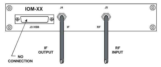
Figure 7. Non-Redundant Converter Configuration
