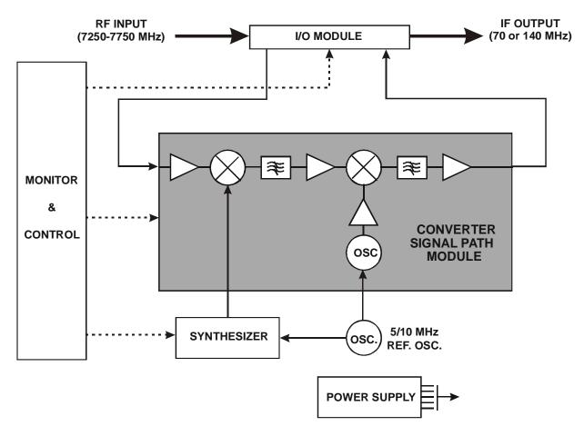
Figure 33. Typical Converter Functional Block Diagram (Model DT-4572 shown)
