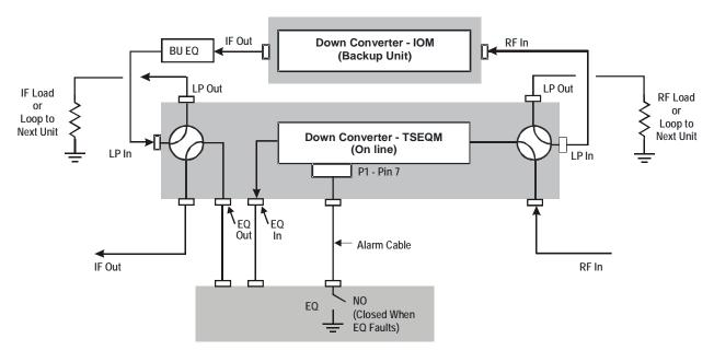
Figure 23. 1:1 Redundant Configuration Diagram - Single Source RF Input with IOM-XX and TSEQM-XX Installed
