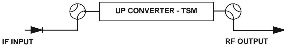
Figure 8. Non-Redundant Converter Configuration With Transmit Switch Module (TSM-XX) Installed
