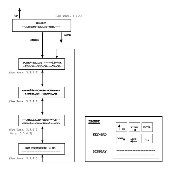
Figure 3-4. Currents Faults Menu Commands
