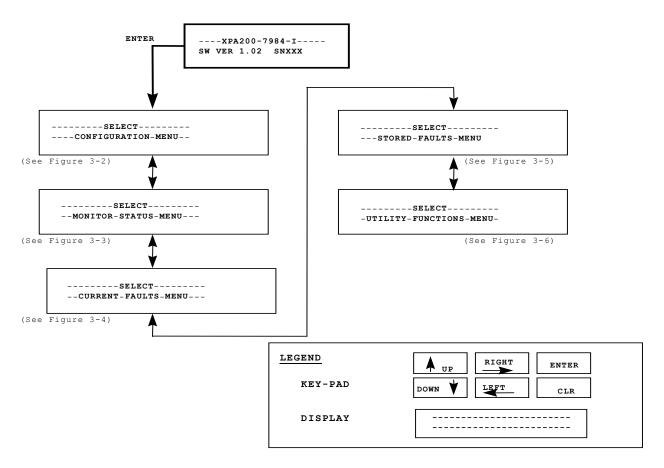
Figure 3-1. SSPA Operating Command Functions
