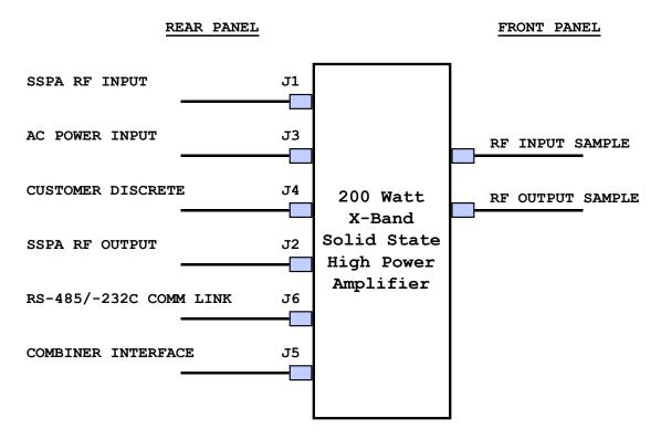
Figure 6-1. SSPA Signal and Interconnecting Cable Diagram
