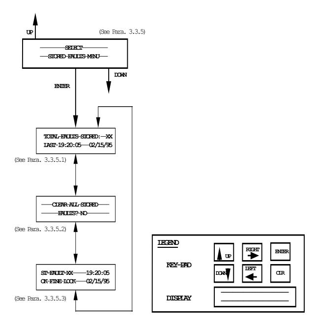
Figure 3-5. Stored Faults Menu Command
