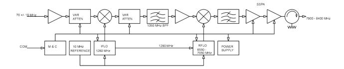
Figure 6-2. Functional Block Diagram of the Upconverter Section
