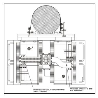
gure 2-23 Waveguide layout
