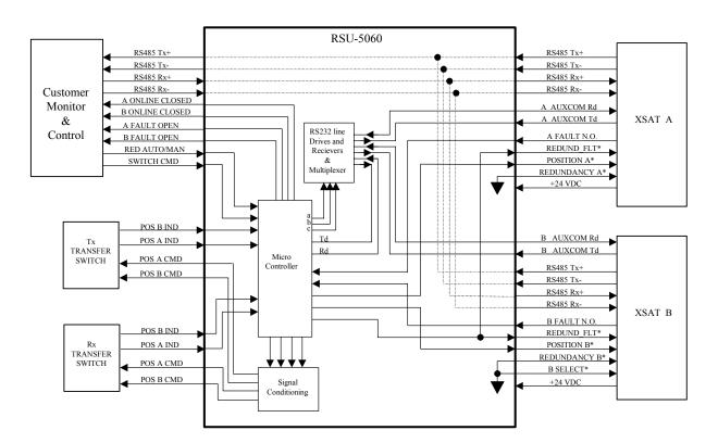
Figure 5-4. RSU-5060 Functional Block Diagram
