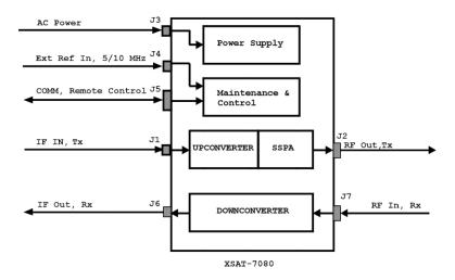
Figure 7-1. Converter Signal and Interconnecting Cable Diagram
