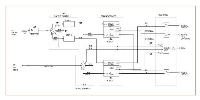
Figure 5-1. Typical XSAT Redundant System, without IF Transfer Switches
