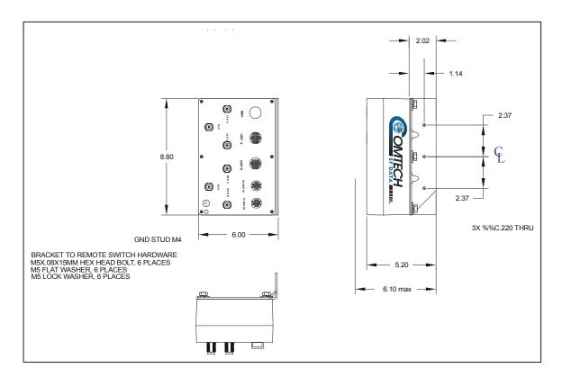
Figure 5-3. Mechanical Dimensions and Mounting Interface
