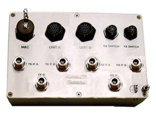
Figure B-15. Remote Switch Box Assembly, AS/0490
