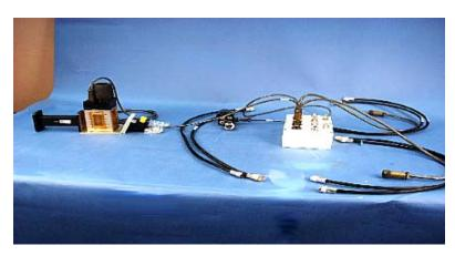
Figure A-17. Remote Switch Cast Box
