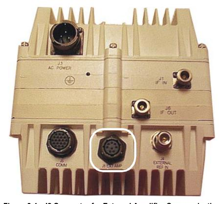
Figure 9-1. J8 Connector for External Amplifier Communication
