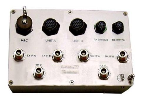
Figure A-14. Assembly, TX/Remote Switch, AS/0490
