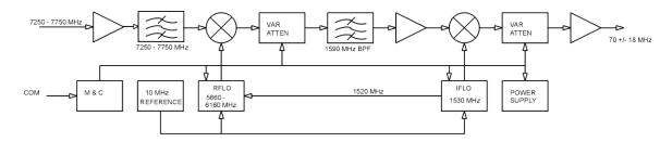
Figure 6-1. Functional Block Diagram of the Downconverter Section
