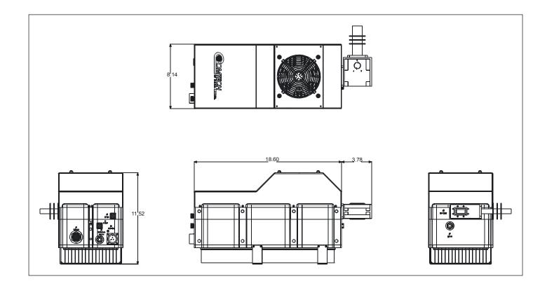
Figure 2-2. 50-WATT Dimensional Drawing
