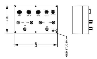
Figure 2-4. Remote Switch Dimensional Drawing
