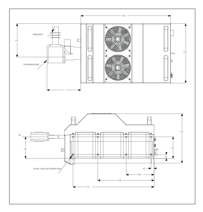
Figure 2-3. 100-WATT Dimensional Drawing
