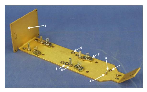
Figure A-10. 1:1 25W XSAT TX Switch Bracket, AS/0489
