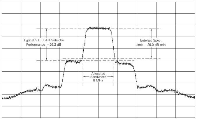
Horizontal Scale 5 MHz/div Vertical Scale 10 dB/div Centre Frequency 14.2 GHz
