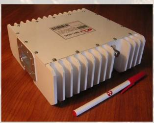
This small and light weight 5W L-To C-Band Block Up Converter is designed to be mounted on the feed horn. High power efficiency resulting in low current (<= 2 amps) consumption allows user to pass DC supply voltage via IF cable. The unit is ideal for network and point to point, data distribution, portable and emergency applications.
