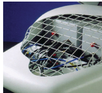
Two HPAs located within the antenna assembly
