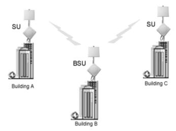
A link between two locations always consists of a Base Station Unit (BSU) and a Subscriber Unit (SU). A BSU can, depending upon its configuration, connect to one or more SUs; an SU, however, can connect to only one BSU.
