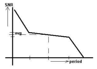
When the antenna is aimed, the beep can easily be heard if the SNR is rising (shorter period, higher frequency) or falling (longer period). When the position of the antenna has been changed, the SNR averaging settles at the new value and the beeping returns to the average length so the antenna can again be aimed towards rising SNR.
