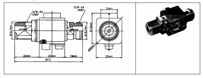
CAUTION! To avoid damage to electronic equipment and your radio equipment, always apply the surge arrestor between the outdoor antenna installation and the radio hardware or other computing device that is connected to the outdoor antennas.
