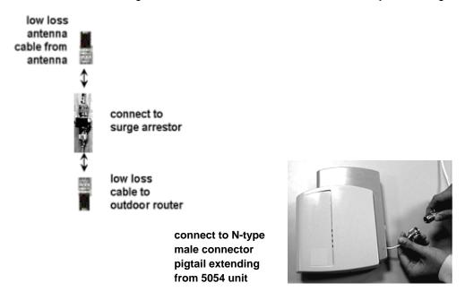
Figure 1. Cable Setup for 5054 Antenna Installation
