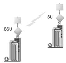
A single point-to-multipoint network, which lets you connect more than two buildings. You can set up a single point-to-multipoint network with a single Base Station Unit and multiple Subscriber Units.
