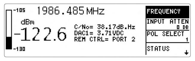
Figure 3-2 Typical Operational Display
